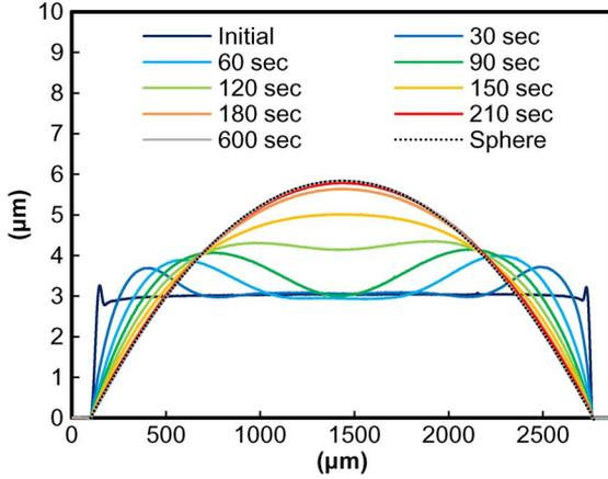
Fig. 3. Reflow of exposed PPC encapsulated by 500 nm of Cu. Profiles correspond to the amount of time that the sample spent on 100 °C hot plate. The stabilized dome matches a spherical cap with a radius of curvature  $R = 15.4$  cm.
