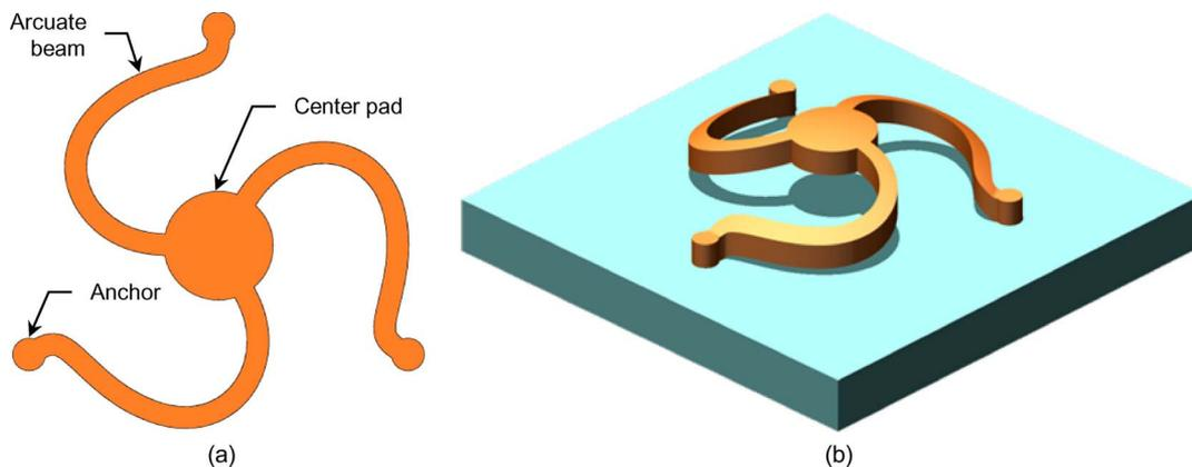
Fig. 10. Domed multipath interconnect design shown as (a) top view and (b) 3-D view on substrate. Similarly as with the thin-film material characterization test, the design features a floating Cu center pad which is anchored to the substrate by three arcuate beams.
