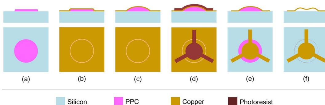
Fig. 6. Fabrication process of test specimen used to characterize the Cu thin-film tensile strength and/or interfacial fracture strength of Cu thin film on Si substrate. The region of the Cu film pattern encompassed by the dotted line in (f) indicates the debonded area.
