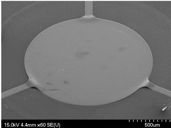
Fig. 8. SEM image showing readhesion of Cu film pattern after PPC decomposition.
