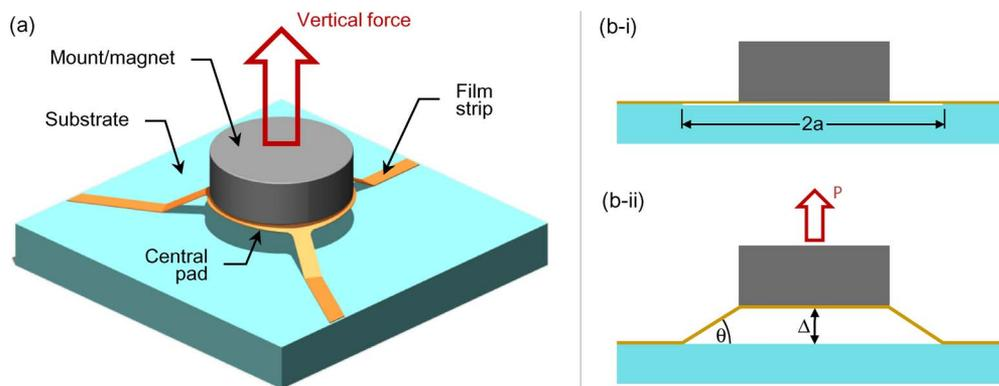
Fig. 5. Thin-film characterization test design. (a) Three-dimensional illustration showing vertical loading of central pad applied through an assembled mount or permanent magnet. Tensile and peeling forces are imposed along the three anchoring film strips. (b) Idealized side view of test specimen showing two anchoring film strips: (i) At rest with initial debonded length  $2a$  and (ii) applied vertical loading with force  $P$ , displacement  $\Delta$ , and strip angle  $\theta$ .
