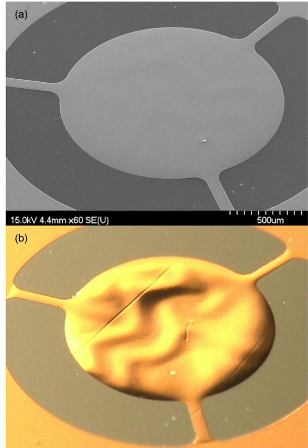
Fig. 9. Released Cu thin-film structure after supercritical drying. The waviness of the released film is too slight to be captured by (a) the SEM but is more visible under (b) an optical microscope.
