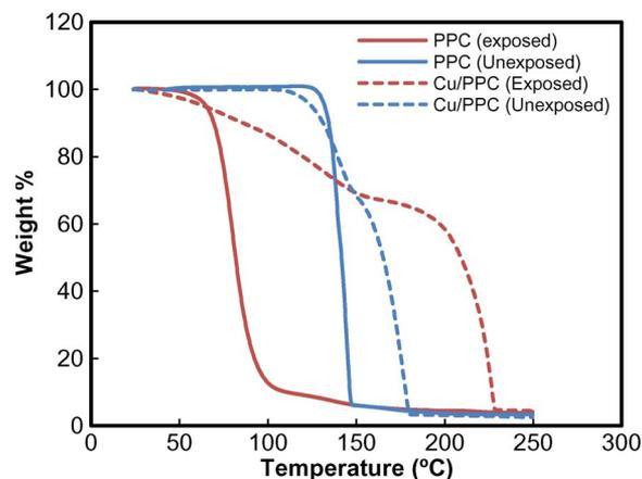
Fig. 7. TGA of exposed/unexposed PPC with and without Cu coating.
