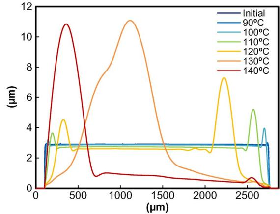
Fig. 2. Reflow of bare unexposed PPC. Profiles correspond to 10 min of heating at each incrementally increasing hot-plate temperature.
