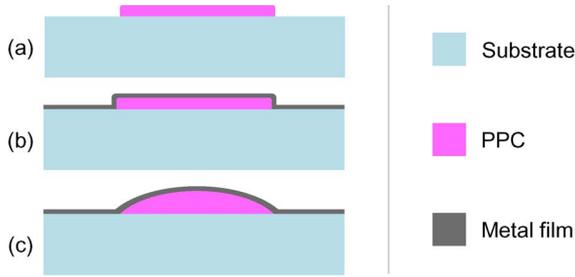
Fig. 1. Fabrication of reflowed polymer domes. (a) PPC patterning. (b) Blanket sputtered metal film. (c) Reflowed PPC on a hot plate into dome shape.
