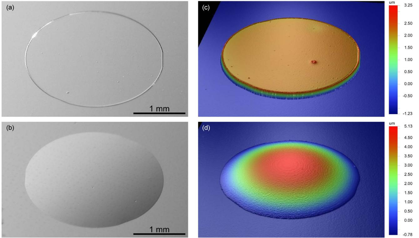
Fig. 4. Cu-coated PPC before and after reflow showing transformation from disk shape to dome shape. (a and b) Optical images taken with Keyence VHX-600 microscope. (c and d) Images generated by Veeco Wyko NT-2000 optical profiler.
