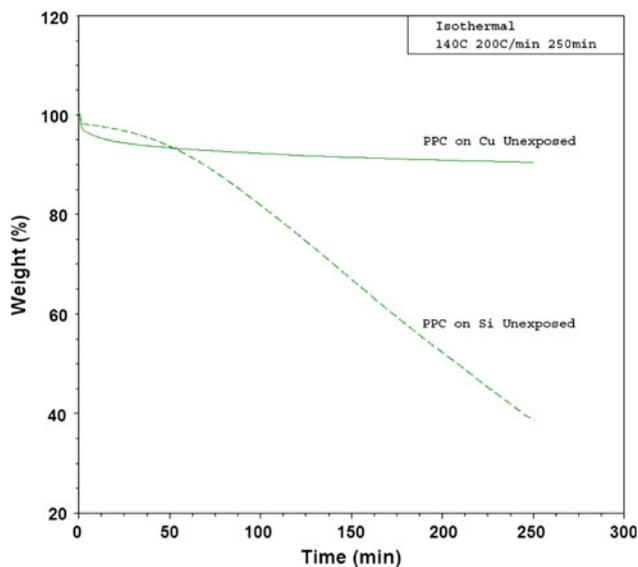
Fig. 6. Isothermal TGA curve at 140°C for a PPC film removed from either silicon or copper substrates without UV exposure.
