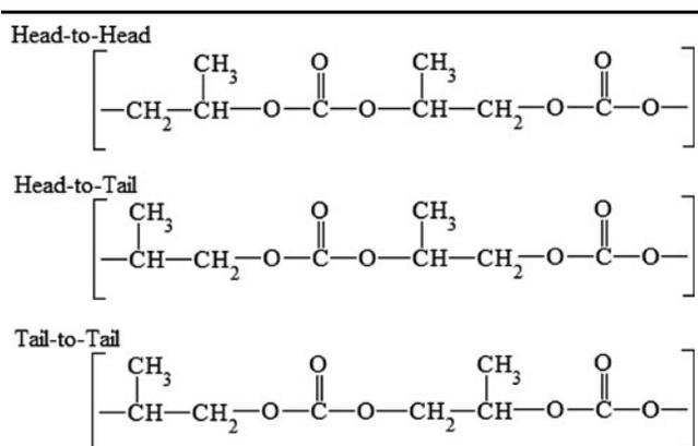
Fig. 1. The local structure of poly(propylene carbonate) can exist as HH, TT or HT. HH and TT are essentially the same structure with a different choice of reference plane. HT is the most desirable, as its alternating structure allows self-propagating decomposition to occur by chain unzipping.
