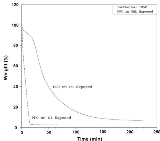
Fig. 5. Isothermal TGA curve at 105°C showing mass fraction versus time for PPC films cast from GBL-dissolved PPC with 3 wt.% PAG on silicon and copper.
