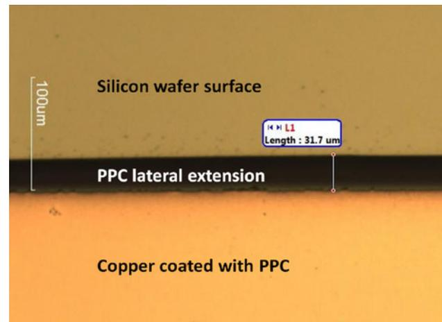
Fig. 11. Plan-view optical microscope image of 31.7  $\mu\text{m}$  PPC lateral extension from copper line edge for PPC film cast from GBL after 3.1 min postexposure bake at 115 $^{\circ}\text{C}$ . The copper line is 17  $\mu\text{m}$  thick on silicon and allows copper uptake from the sidewall into PPC.
