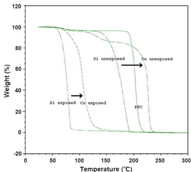
Fig. 3. Dynamic TGA plots for PPC films in GBL cast on a copper surface (exposed to copper) and cast on silicon (not exposed to copper) with and without UV exposure compared with decomposition of neat PPC without UV exposure.
