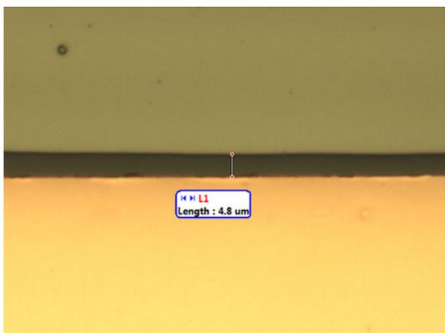
Fig. 14. Plan-view optical microscope image of 3.9  $\mu\text{m}$  PPC lateral extension from copper line edge for PPC film cast from MeCl after 3.0 min postexposure bake at 98°C. Residue due to incomplete decomposition extends 10  $\mu\text{m}$  from copper line edge.
