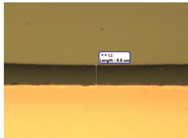
Fig. 12. Plan-view optical microscope image of 9.8  $\mu\text{m}$  PPC lateral extension from copper line edge for PPC film cast from MeCl after 70 min postexposure bake at 78 $^{\circ}\text{C}$ .
