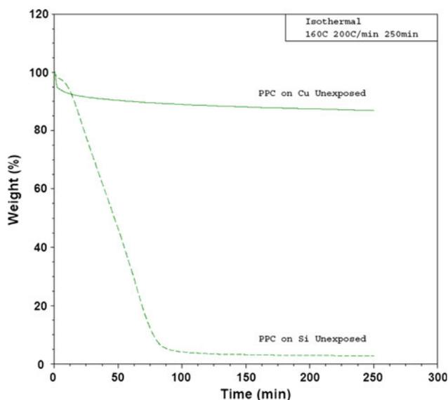
Fig. 7. Isothermal TGA curve at 160°C for a PPC film removed from either silicon or copper substrates without UV exposure.
