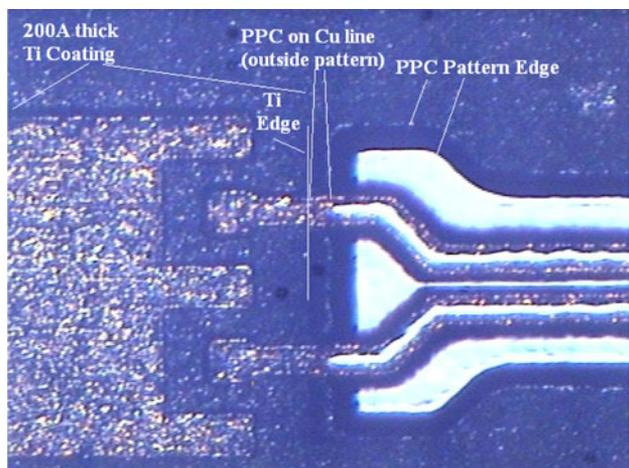
Fig. 18. Optical microscope image of copper probe pads coated with titanium to prevent PPC self-patterning. The titanium barrier layer prevents uptake of copper into PPC, disabling the self-patterning characteristics. As in Fig. 17, the white region is PPC and is masked to form the dog-bone shape encapsulating the copper lines. The copper on the left side of the image has been coated with 200 Å of Ti prior to PPC spin-coating and patterning.
