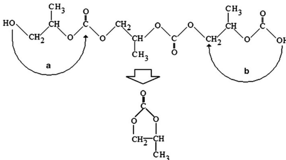
Fig. 2. Chain unzipping of an acid-activated termination can proceed via (a) alkoxide biting or (b) carbonate biting. Both mechanisms yield cyclic propylene carbonate as the primary product with fragment products of carbon dioxide, acetone, and other low-molecular-weight species.
