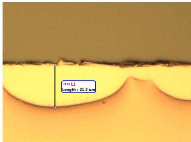
Fig. 15. Plan-view optical microscope image of 21.2  $\mu\text{m}$  PPC retraction from copper line edge for PPC film cast from TCE after 3.0 min postexposure bake at 100°C.
