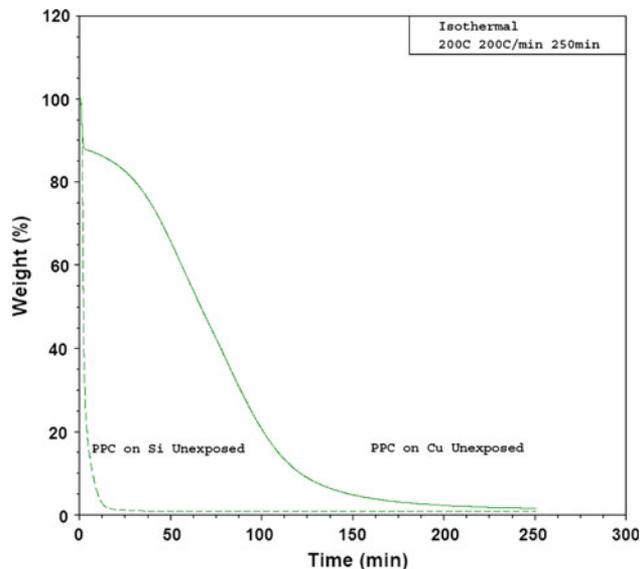
Fig. 8. Isothermal TGA curve at 200°C for a PPC film removed from either silicon or copper substrates without UV exposure.
