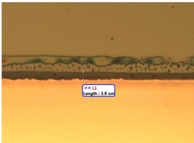
Fig. 13. Plan-view optical microscope image of 4.8  $\mu\text{m}$  PPC lateral extension from copper line edge for PPC film cast from TCE after 41 min postexposure bake at 80°C.
