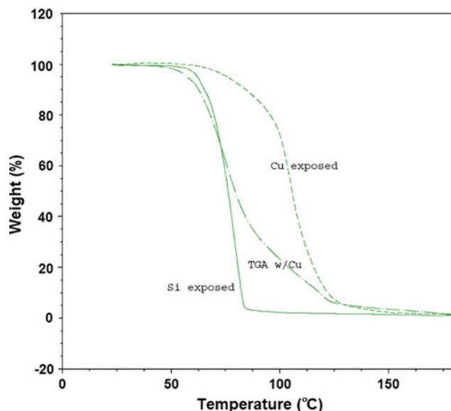
Fig. 4. Dynamic TGA plots for exposed PPC films on copper and silicon substrates cast from solutions dissolved in GBL. Samples were exposed to 1 J/cm<sup>2</sup> UV at  $\lambda = 248$  nm and decomposed in nitrogen at a heating rate of 0.5°C/min. The curve labeled “with Cu” was cast from TCE (no GBL) and had copper mixed with the polymer material during the TGA experiment.
