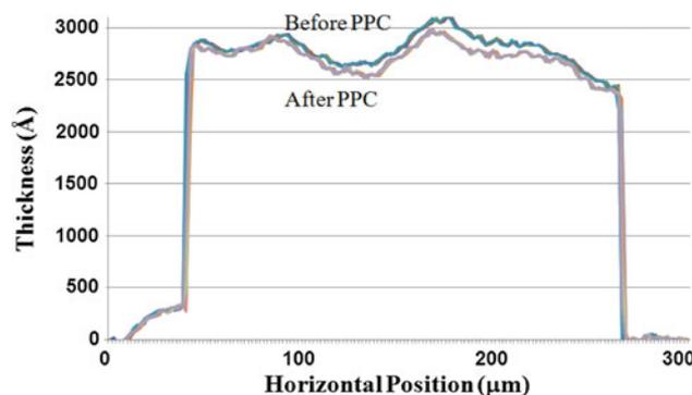
Fig. 16. Copper removed from line surface by copper. Shown are surface profiles of a copper line before coating with PPC and after stripping PPC. The average thickness removed from the copper line surface between 150  $\mu\text{m}$  and 850  $\mu\text{m}$  was 67 Å and is used for calculations shown in Table I.
