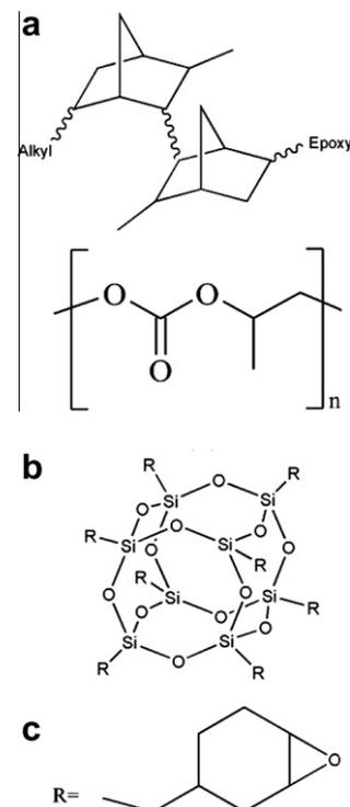
**Fig. 3.** Chemical structures of polymers used in fabrication. (a) Avatrel 2000P, (b) polypropylene carbonate and (c) epoxy cyclohexyl POSS.
