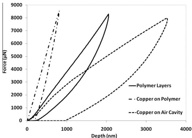
**Fig. 10.** Force versus displacement curves using a cono-spherical tip with a maximum force of 8750  $\mu\text{N}$  for a fully constructed polymer field (solid line), copper line in the polymer field (dot-dashed line), and the copper line on the air cavity (dashed line).
