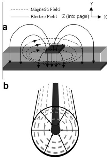
**Fig. 1.** Schematic of electrical and magnetic fields for a transmission line. (a) Microstrip transmission line and (b) coaxial transmission line.
