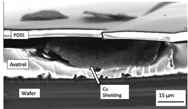
Fig. 7. SEM image of a cross-sectioned decomposed half coaxial air cavity. The crack in the POSS cavity is due to excessive cavity pressure during decomposition.
