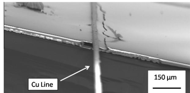
Fig. 8. SEM image of a cross-sectioned half coaxial transmission line. The copper transmission line extends beyond the sample. The crack in the POSS overcoat is due to cross-sectioning of the sample.
