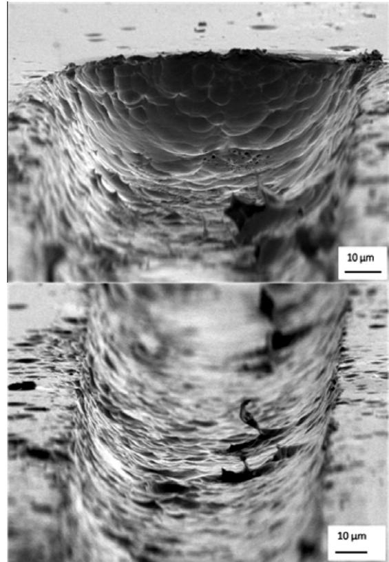
Fig. 5. SEM images of the semi-circular trench imprinted in Avatrel 2000P at 110 °C, 45 bar for 60 s.
