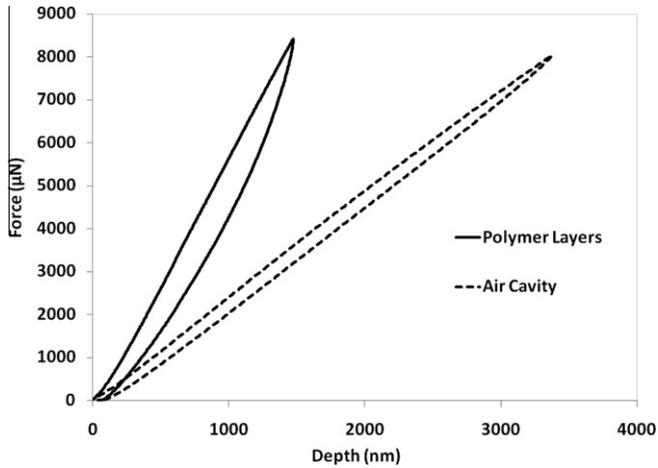
**Fig. 9.** Force versus displacement curves using a cono-spherical tip with a maximum force of 8750  $\mu\text{N}$  for a fully constructed polymer field (solid line) and a POSS over-coated air cavity (dashed line).
