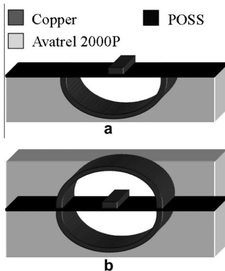
**Fig. 2.** Schematic of constructed (a) half-coaxial and (b) air-clad coaxial transmission line.
