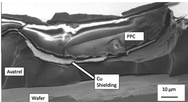
Fig. 6. SEM image of a cross-sectioned, copper-clad, semi-circular trench with patterned PPC in trench and a layer of gold for imaging.
