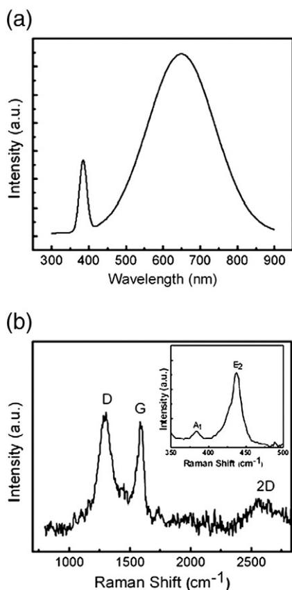
**Fig. 3.** (a) Photoluminescence and (b) Raman spectra of ZnO NRs directly grown on the CCG film with dots.
