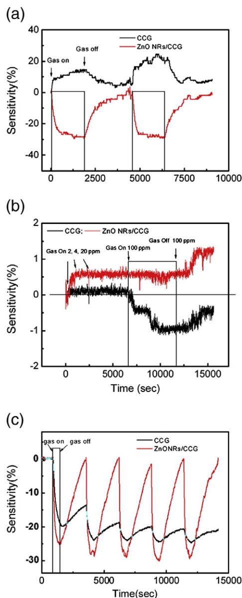
**Fig. 4.** The sensitivity of ZnO NRs-CCG sensors to  $H_2S$  gas in (a) oxygen at RT and (b) nitrogen at RT, and (c) nitrogen at  $270\text{ }^\circ\text{C}$ .
