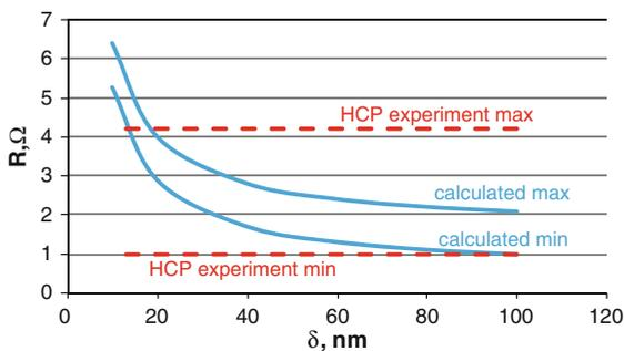
**Fig. 12** HCP hypothesis: Calculated and experimental margins for total measured resistance
