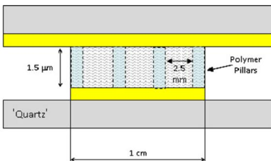
**Fig. 4** GCM-3 polymer pillar gap control method
