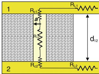
**Fig. 8** Electrical schematic for the test cell
