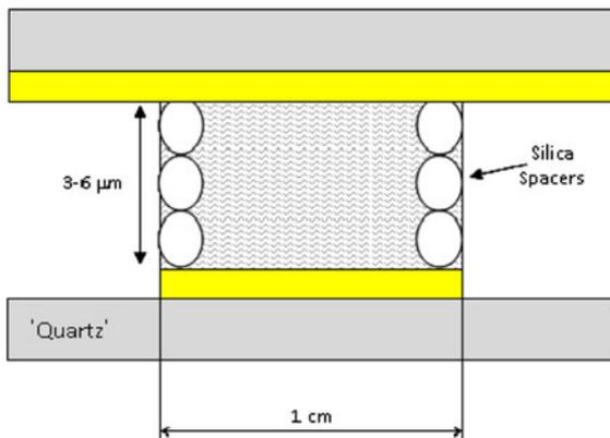
**Fig. 3** GCM-2 silica particle gap control method
