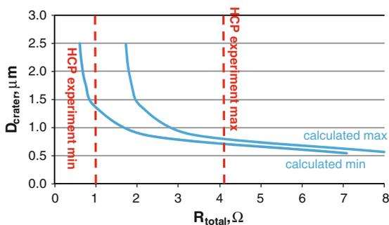
**Fig. 11** Metal filament hypothesis: Crater diameter as a function of resistance
