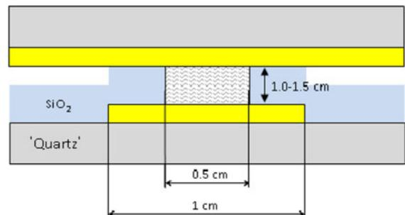
**Fig. 2** GCM-1 silicon dioxide gap control method
