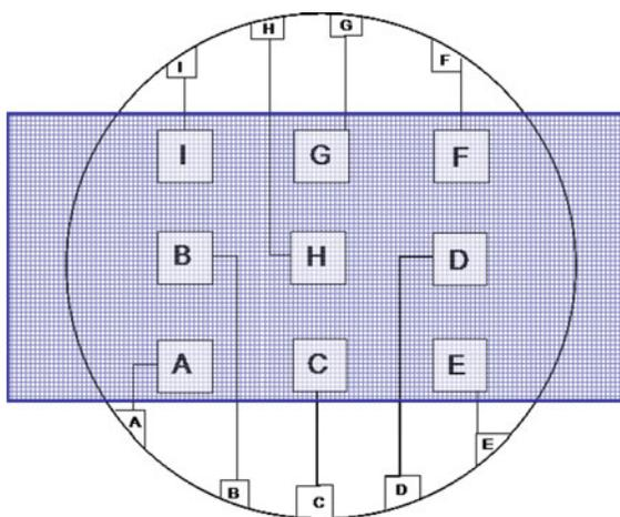
**Fig. 1** Bottom (round wafer) and top (rectangular, blue) electrode set-up
