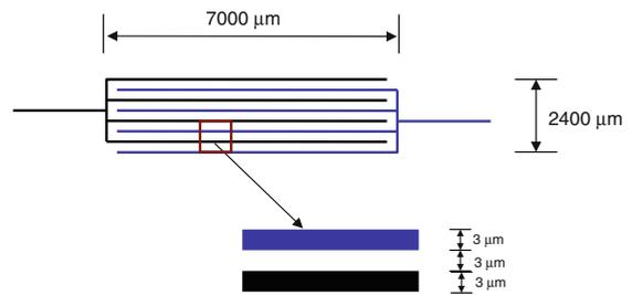
**Fig. 5** Comb electrode schematic
