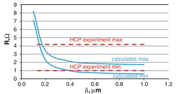
**Fig. 9** Metal filament hypothesis: Calculated and experimental margins for total measured resistance
