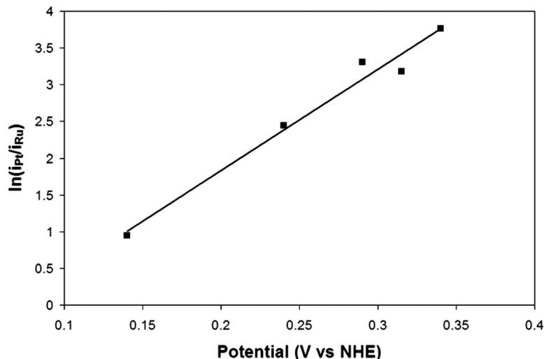
**Fig. 1 Relative contributions to the observed current of Pt and Ru during electrodeposition as a function of potential at 23 °C and  $C_{Pt}/C_{Ru}=1.6$**
