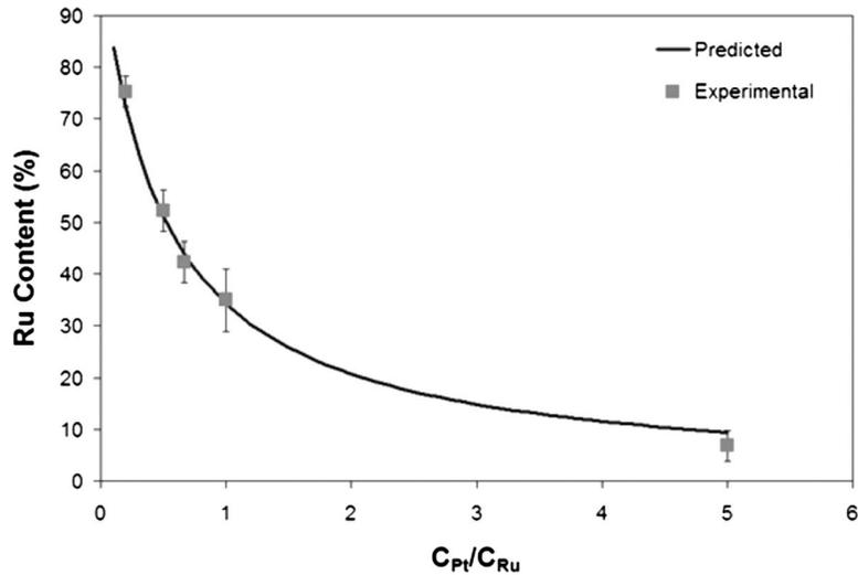
Fig. 5 Model and experimental results for the electroless deposition of  $Pt_xRu_{1-x}$  with formic acid reducing agent and various bath compositions ( $70^\circ\text{C}$ )
