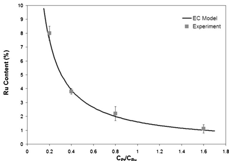
**Fig. 3 Agreement between the proposed deposition model at a surface potential of  $0.4$  V and experimental data for the spontaneous, electroless deposition of Pt<sub>x</sub>Ru<sub>1-x</sub> with a hydrazine dihydrochloride reducing agent at various bath compositions (23°C).**
