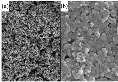
**Fig. 2 Anode catalyst layer (a) before and (b) after the electroless deposition of PtRu at 11,000 $\times$  and 60,000 $\times$  magnifications, respectively**
