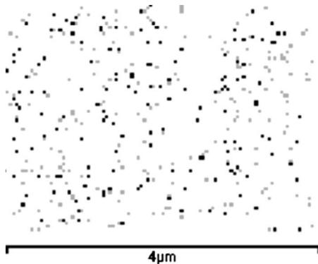
Fig. 6 EDX map for Pt (■) and Ru (□) in the  $Pt_{0.48}Ru_{0.52}/C-SiO_2$  composite catalyst layer
