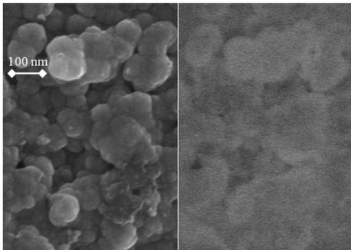
Fig. 7 SEM/backscatter SEM for PtRu catalyst layer, 125 kx magnification (100 nm marker shown)
