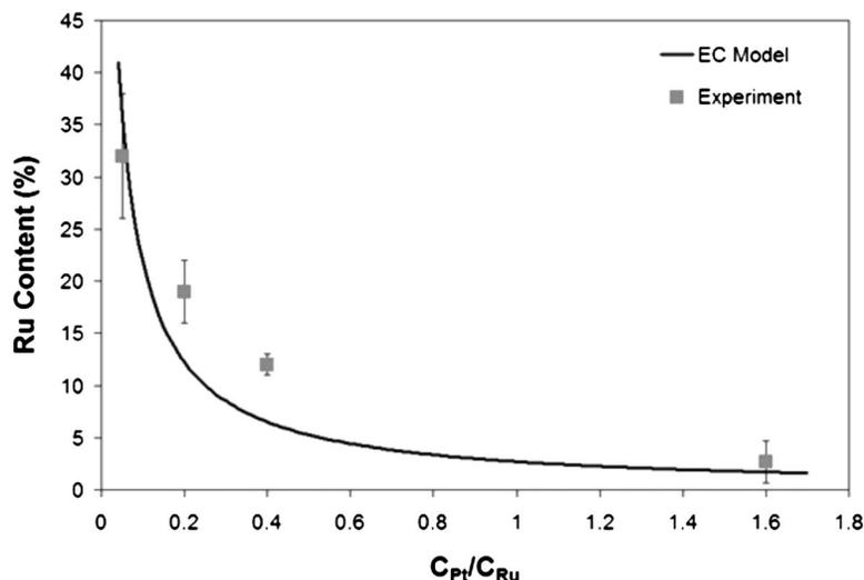
**Fig. 4 Model and experimental results for the electroless deposition of  $Pt_xRu_{1-x}$  with hydrazine dihydrochloride reducing agent and various bath compositions (90 °C)**
