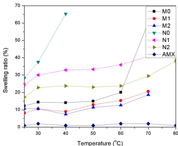
Fig. 7. Temperature dependence of swelling ratio of the different membranes.
