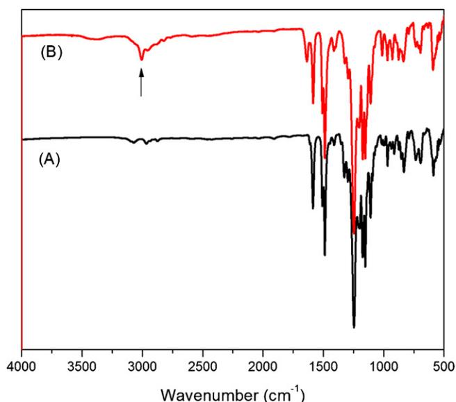
**Fig. 3.** FT-IR spectra of crosslinked CMPSF/4EP (A) and aminated crosslinked (B) membranes.
