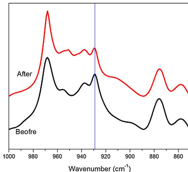
Fig. 2. Comparison of the FT-IR spectra of before and after thermally cured CMPSF/4EP membranes.
