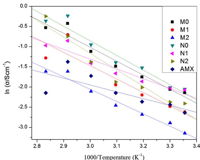
Fig. 9. The  $\ln \sigma$  vs.  $1000/T$  plot for the different membranes; the lines indicate the linear regression.
