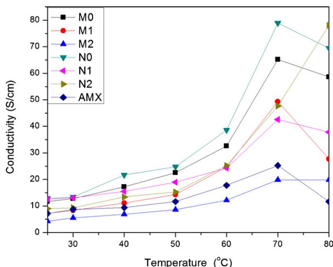
Fig. 8. Temperature dependence of the ionic conductivity of the different membranes.
