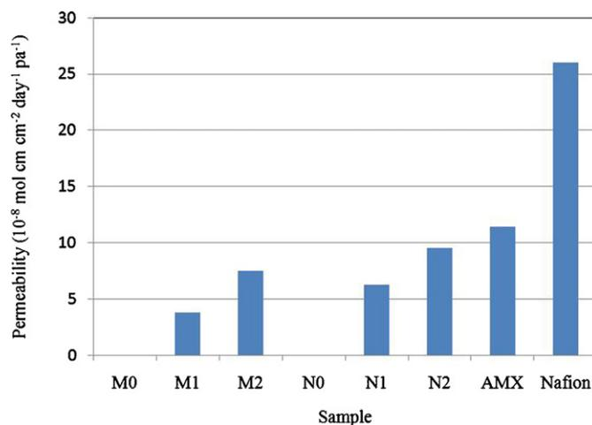
Fig. 10. Methanol permeability of different membranes at room temperature.
