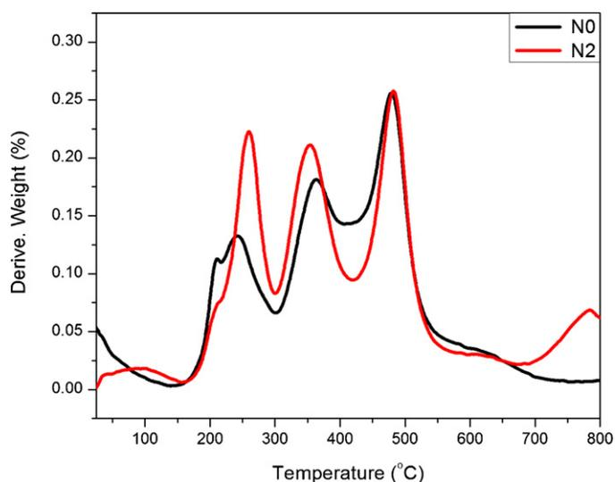
**Fig. 5.** DGA curves of non-crosslinked (N0) and crosslinked membranes (N2) in nitrogen.
