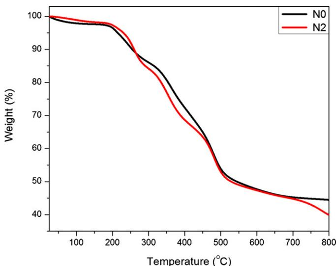
**Fig. 4.** TGA curves of non-crosslinked (N0) and crosslinked membranes (N2) in nitrogen.
