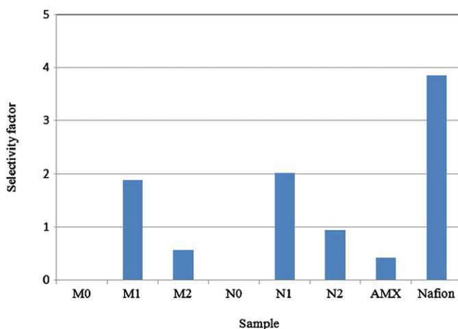
Fig. 11. Selectivity factor of different membranes at room temperature.
