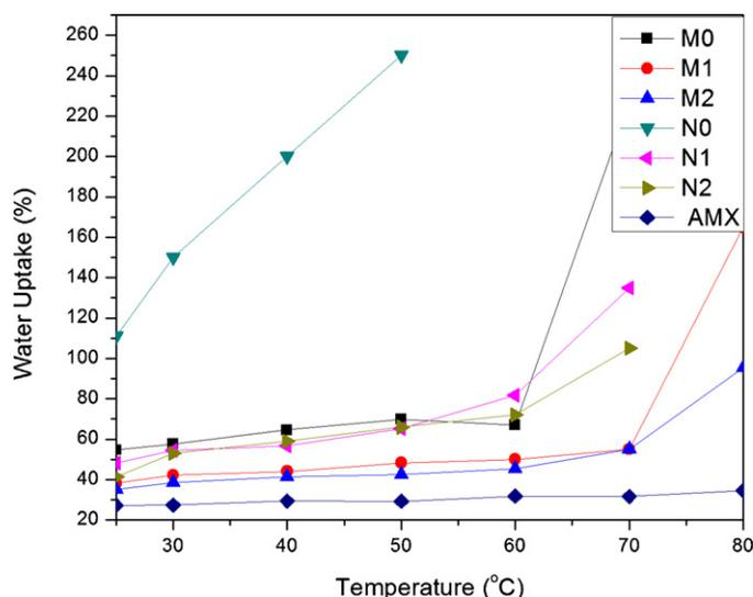
Fig. 6. Temperature dependence of water uptake of the different membranes.
