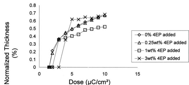
FIG. 9. Unity<sup>®</sup> 4671E thickness measured over a dose range with different concentrations of 4EP added.
