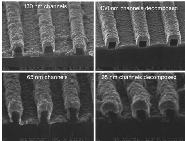
FIG. 10. 65 and 130 nm nanochannels before and after decomposition.
