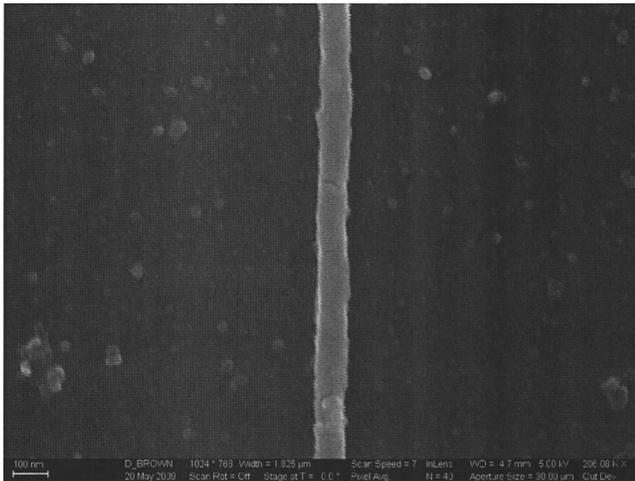
FIG. 5. PECVD oxide coating of a 500 nm line of Unity with no decomposition.
