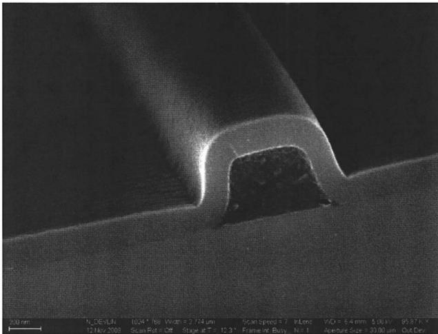
FIG. 6. PECVD oxide coating after Unity decomposed by furnace creating 500 nm channels.
