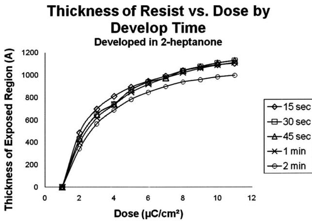
FIG. 2. Unity® 4671E thickness measured over a dose range with four different developers.
