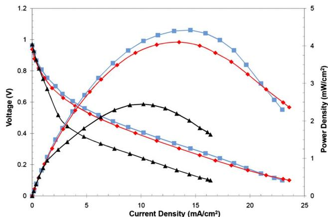
**Figure 2.** (Color online) Polarization curves of the same MEA for the cathode stream with (▲) humidified O<sub>2</sub> (test 1), (●) humidified O<sub>2</sub> + CO<sub>2</sub> (test 2), and (■) dry O<sub>2</sub> + CO<sub>2</sub> (test 3). The anode feed is humidified H<sub>2</sub> in all conditions.
