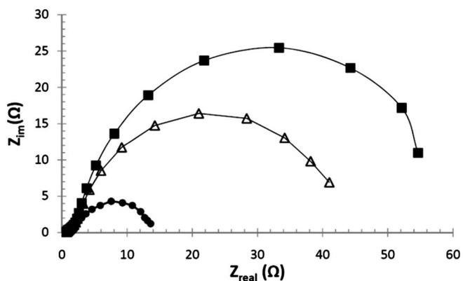
Figure 5. EIS spectra at (■) 800, (△) 700, and (●) 300 mV for test 2 conditions.
