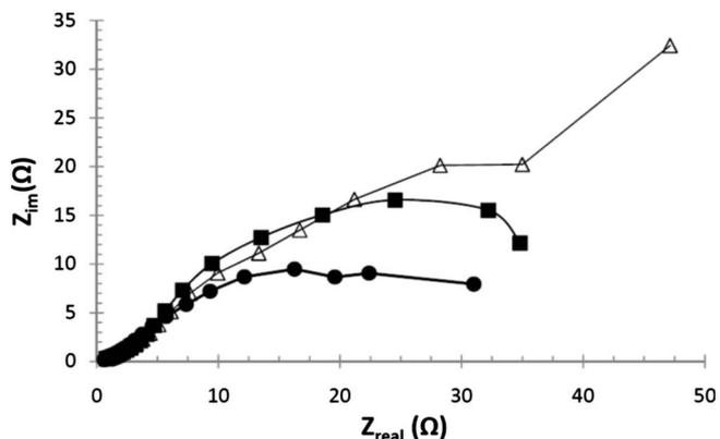
Figure 4. EIS spectra at (■) 800, (△) 700, and (●) 300 mV for test 1 conditions.
