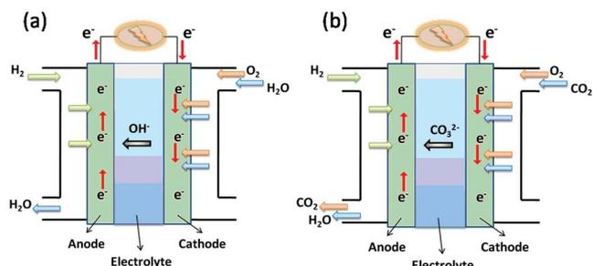
**Figure 1.** (Color online) Diagram of fuel cells operating on (a) the hydroxide cycle and (b) the carbonate cycle.
