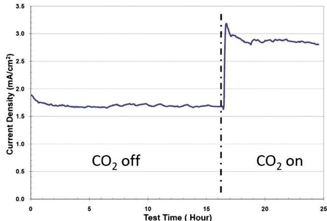
**Figure 3.** (Color online) Current density of fuel cell operating at 600 mV and 25°C with and without CO<sub>2</sub> in the cathode stream. The anode feed is humidified H<sub>2</sub>.
