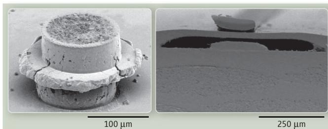
**Better interconnects.** (Left) Two copper pillars joined through an electroless fusion process. (Right) Cross section of air-isolated microstrip line.
