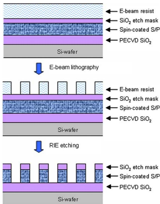
Fig. 3. The fabrication processes of sacrificial polymer lines, 50 nm in width and 85 nm in height.
