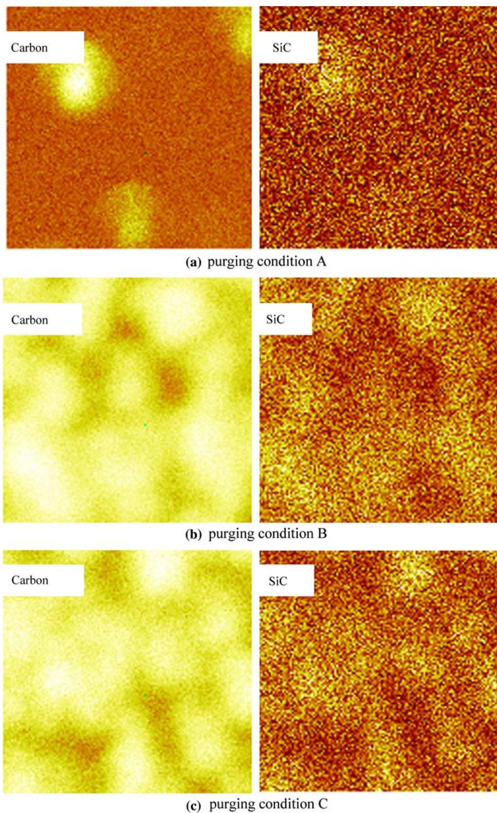
Fig. 10. TOF-SIMS carbon and SiC elemental mapping images of decomposition residues of TD-based sacrificial polymer: (a) purging condition A, (b) purging condition B, and (c) purging condition C. Each image is a 1  $\mu\text{m}$  field.
