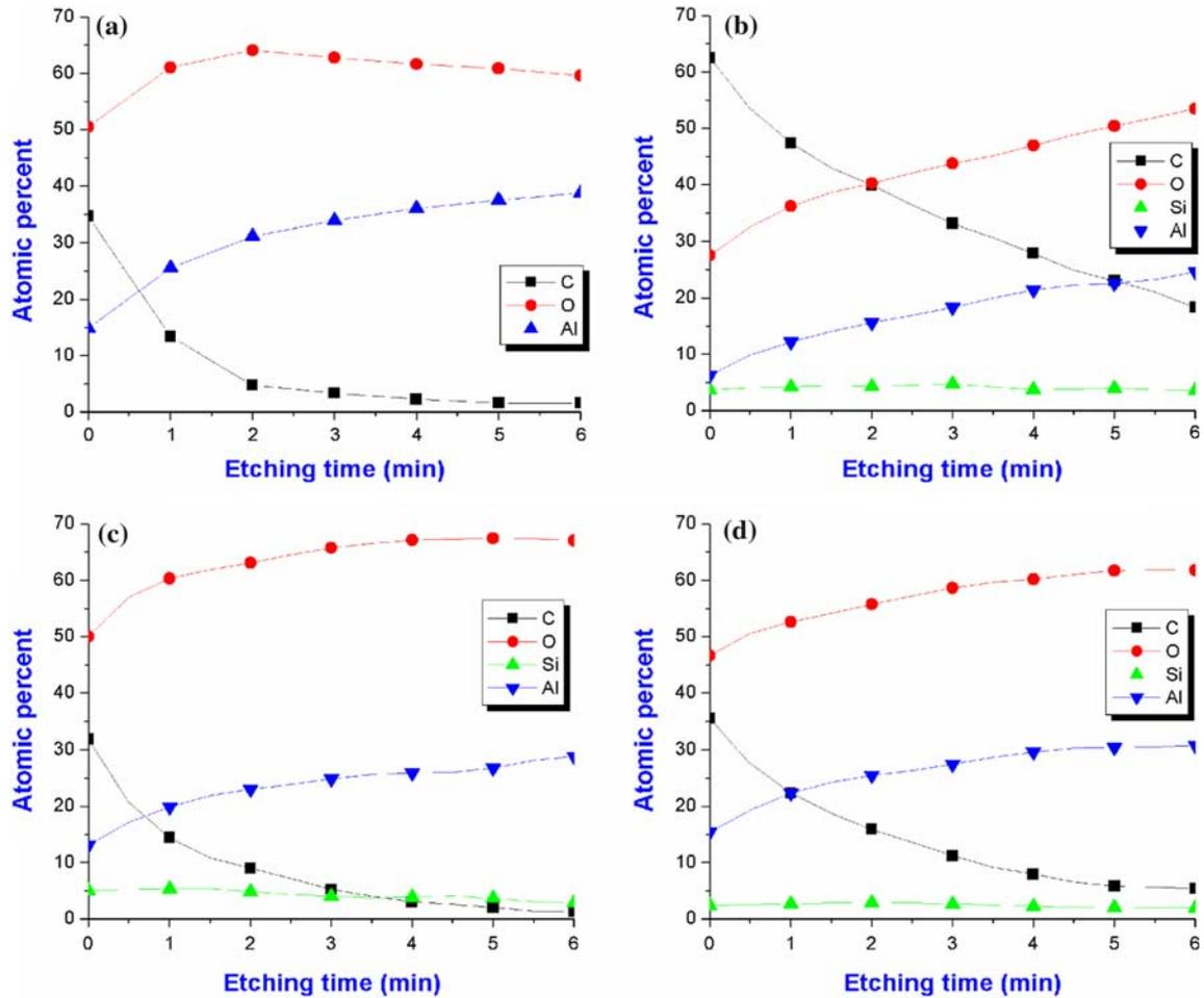
Fig. 9. XPS depth profiling of the decomposition residues of a TD-based sacrificial polymer with different purging conditions during the thermal decomposition: (a) bare Al on Si-wafer, (b) purging condition A, (c) purging condition B, and (d) purging condition C.
