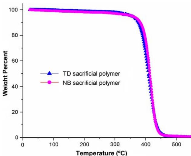
Fig. 8. Dynamic TGA of TD- and NB-based sacrificial polymers.
