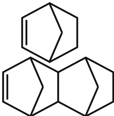
Fig. 2. The chemical structures of monomer units of (a) norbornene (NB) and (b) tetracyclododecene (TD) sacrificial polymers.
