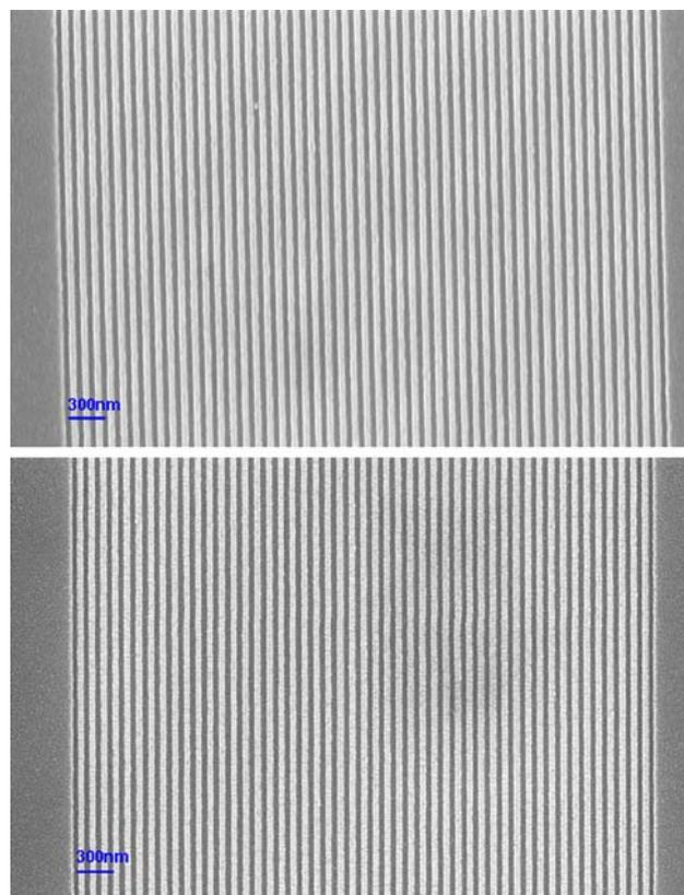
Fig. 6. Top view scanning electron microscopic images of the patterns of SiO<sub>2</sub> hard mask on top of hard-baked sacrificial polymer layers.
