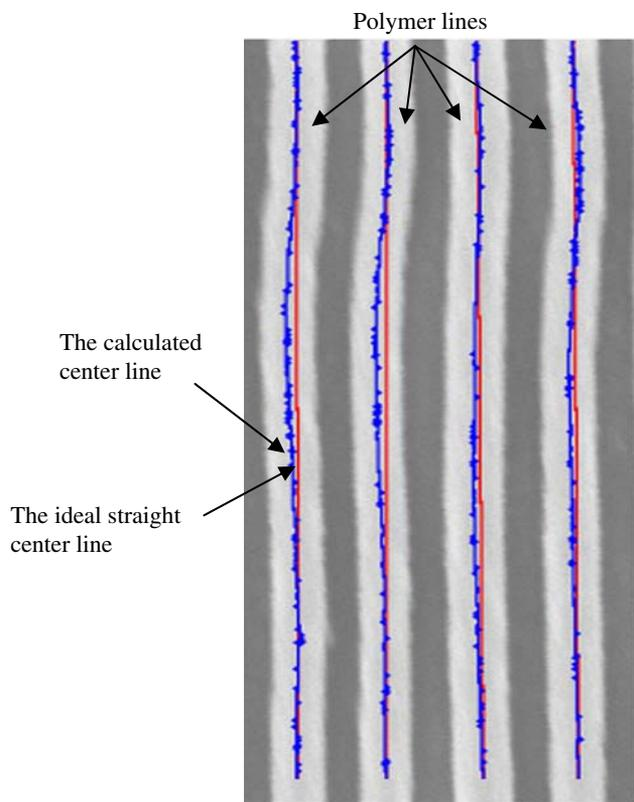
Fig. 5. Sample image to determine the ideal straight center lines and the calculated center lines reflecting the actual shapes of polymer lines, NB-based sacrificial polymer, RF power = 300 W. Each line and space is 50 nm.
