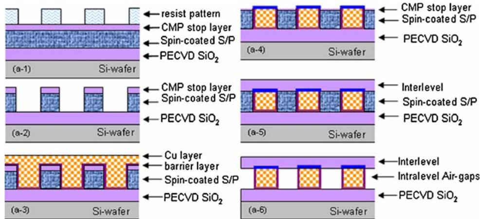
Fig. 1. Schematic diagram of the fabrication process of the single-layer Cu/air-gap interconnect structure.
