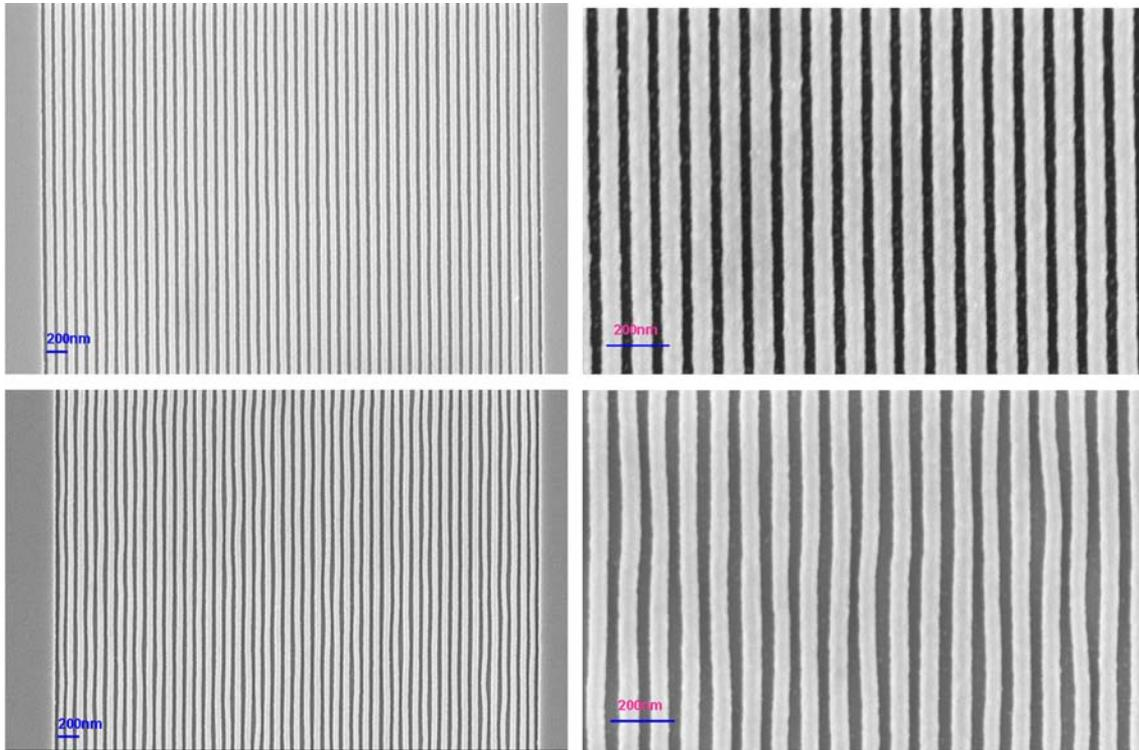
Fig. 7. Top view scanning electron microscopic images of the lines of TD- and NB-based sacrificial polymers, RF power = 400 W.
