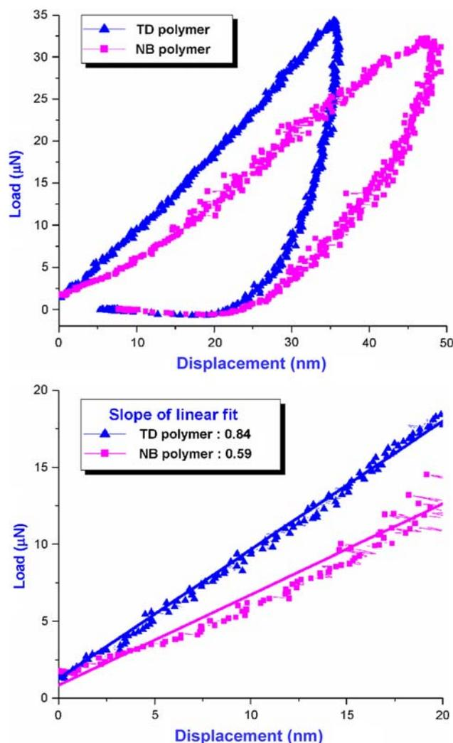
Fig. 4. The load–displacement curves of thin films of TD- and NB-based sacrificial polymers using a nanoindenter.
