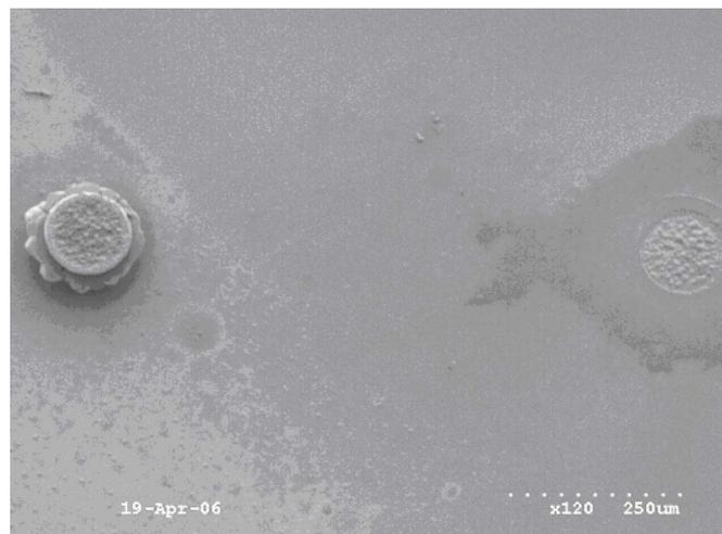
Figure 3. SEM picture of a sheared off substrate.
