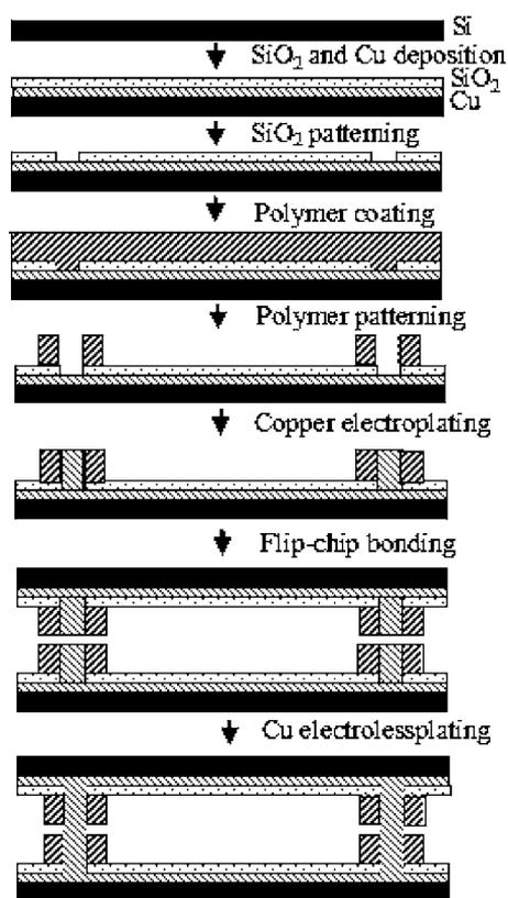
Figure 1. Fabrication process flow.
