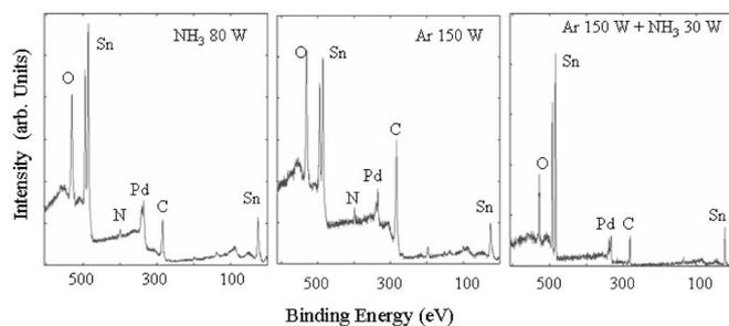
**Figure 8.** XPS survey scans of  $\text{NH}_3$  80 W, Ar 150 W, and Ar 150 W +  $\text{NH}_3$  30 W plasma treated PI samples after the Sn-Pd activation step.
