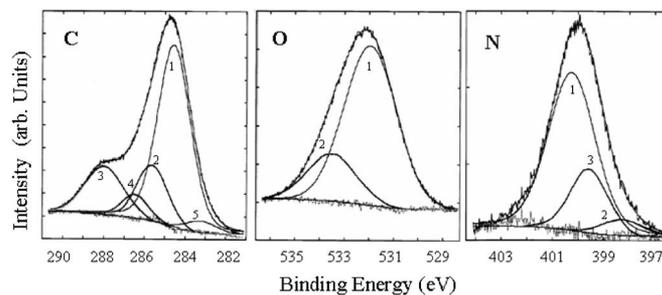
**Figure 6.** C, O, and N core-level XPS spectra after 150 W Ar plasma treatment.
