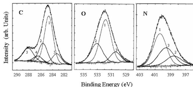
**Figure 5.** C, O, and N core-level XPS spectra after 80 W NH<sub>3</sub> plasma treatment.
