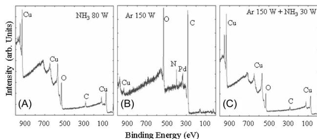
**Figure 13.** XPS survey scans after 5 s electroless Cu deposition for different plasma treatments: (A)  $\text{NH}_3$  80 W; (B) Ar 150 W; and (C) Ar 150 W +  $\text{NH}_3$  30 W.
