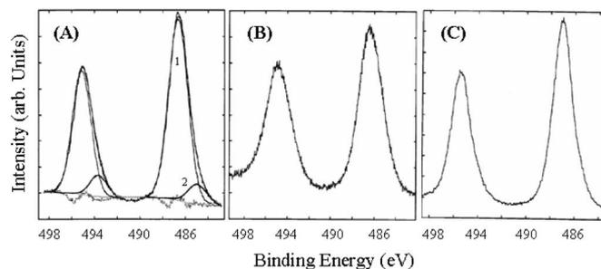
**Figure 9.** Core-level XPS spectra of Sn on PI surface with three different plasma treatments: (A)  $\text{NH}_3$  80 W; (B) Ar 150 W; and (C) Ar 150 W +  $\text{NH}_3$  30 W.
