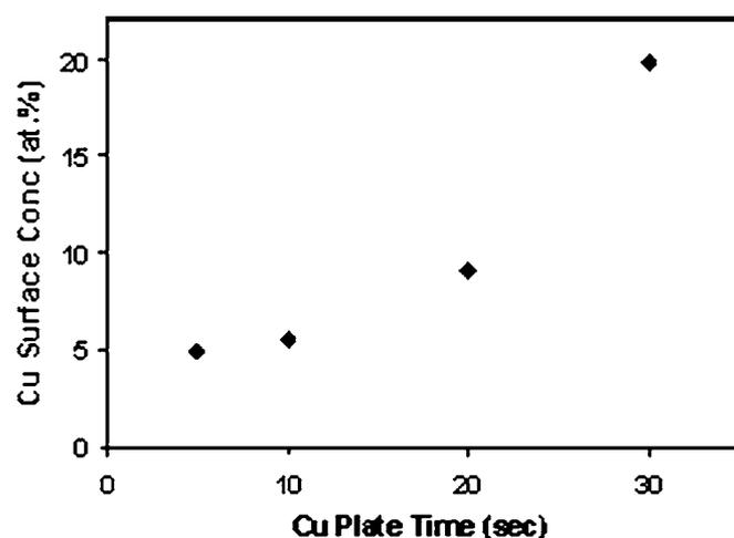
Figure 15. Progression of Cu surface coverage of the  $\text{NH}_3$  30 W sample with electroless plating time.
