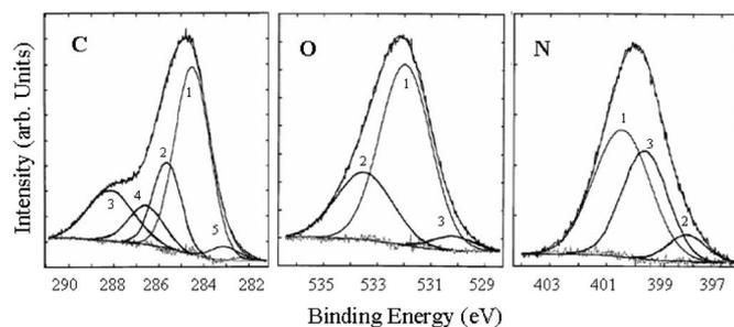
**Figure 7.** C, O, and N core-level XPS spectra after combined plasma treatment with 150 W Ar followed by 30 W  $\text{NH}_3$ .
