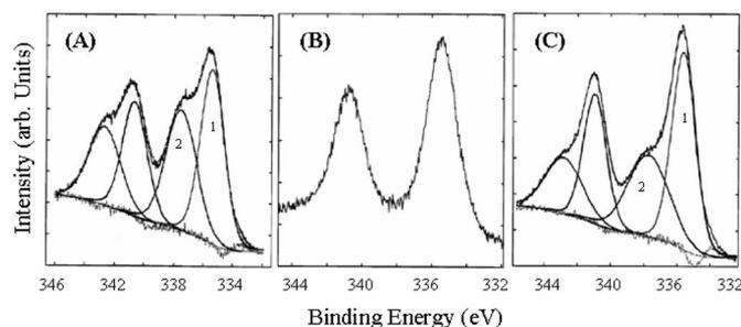
**Figure 10.** Core-level XPS spectra of Pd on PI surface with three different plasma treatments (A)  $\text{NH}_3$  80 W; (B) Ar 150 W; and (C) Ar 150 W +  $\text{NH}_3$  30 W.
