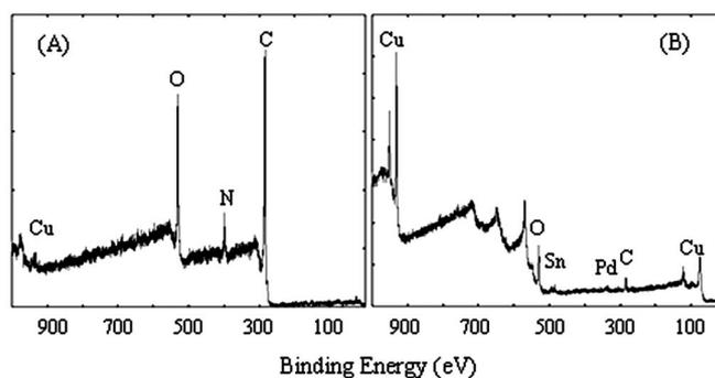
Figure 17. XPS analysis of the (A) PI and (B) Cu surfaces after peeling the Cu film.
