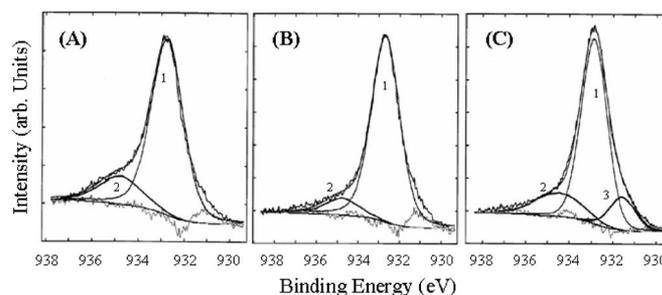
**Figure 14.** Core-level XPS spectra of Cu on PI surfaces with different plasma treatments: (A)  $\text{NH}_3$  80 W; (B) Ar 150 W; and (C) Ar 150 W +  $\text{NH}_3$  30 W.
