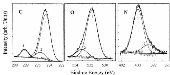
**Figure 4.** Core-level XPS spectra of C, O, and N in untreated PI films.
