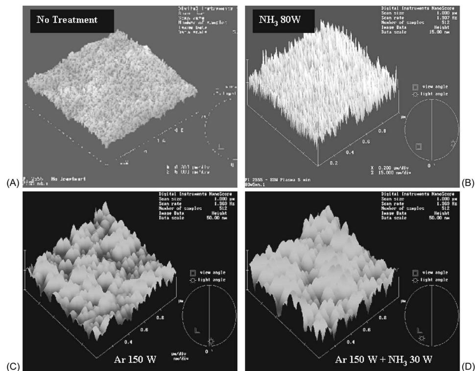
**Figure 2.** Variations in the surface roughness of PI films with different plasma treatments (A) No treatment:  $R_{\text{rms}} = 4.2 \text{ \AA}$ ; (B)  $\text{NH}_3$  80 W:  $R_{\text{rms}} = 29.3 \text{ \AA}$ ; (C) Ar 150 W:  $R_{\text{rms}} = 175.5 \text{ \AA}$ ; and (D) Ar 150 W +  $\text{NH}_3$  30 W:  $R_{\text{rms}} = 183.2 \text{ \AA}$ .
