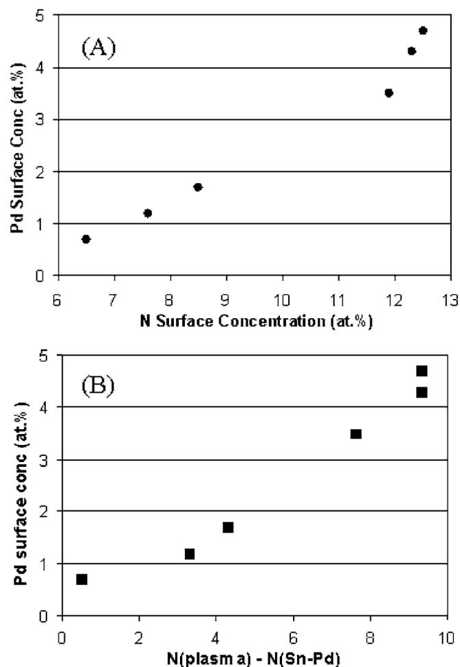
**Figure 11.** Correlation between (A) N surface concentration and amount of Pd adsorbed and (B) reduction in N surface concentration and amount of Pd adsorbed.
