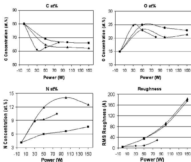
**Figure 3.** Variations in the surface concentrations of C, O, and N and surface roughness of the PI films with plasma power ( $\blacklozenge$ -NH<sub>3</sub> plasma,  $\blacksquare$ -Ar plasma, and  $\blacktriangle$ -Ar + NH<sub>3</sub> plasma).
