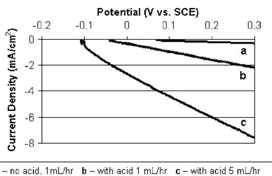
Figure 6. Half-cell performance of microchannels with methanol-water and acid-methanol-water solutions.
