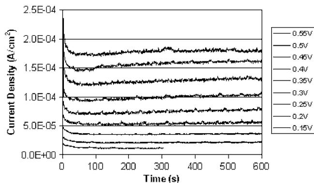
Figure 10. Current density of the imbedded catalyst sample held at constant potential for 10 min.
