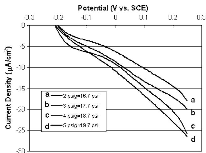
Figure 5. Half-cell performance of microchannels with humidified hydrogen.
