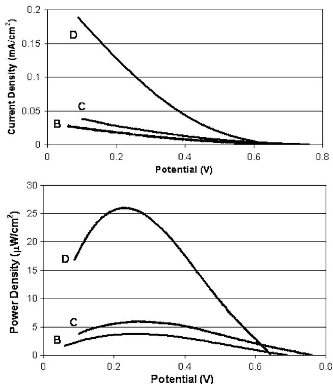
Figure 9. Ambient temperature microfuel cell performance for samples B, C, and D with different amounts of sputtered anode catalyst.
