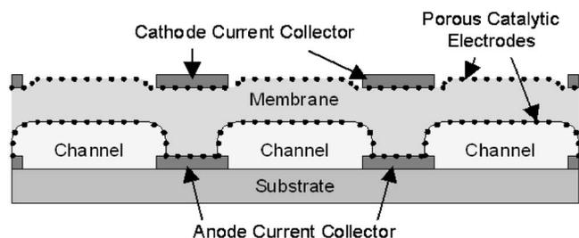
Figure 2. Cross section of a thin-film fuel cell with parallel microchannels.
