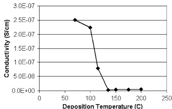
Figure 4. Ionic conductivity of  $\text{SiO}_2$  films measured through impedance spectroscopy.
