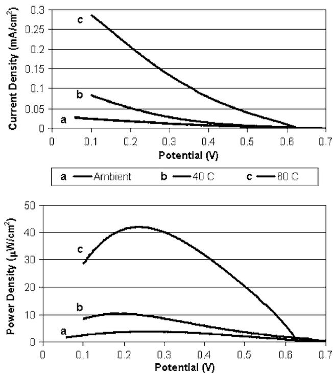
Figure 8. Microfuel cell performance with sputtered anode and thick-film cathode.
