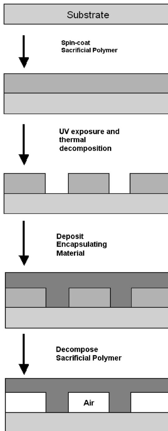
Figure 1. Microchannel formation process using photodefinable PPC.
