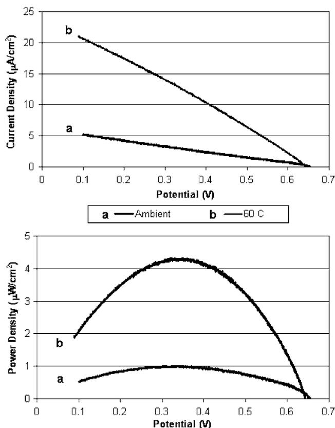
Figure 7. Microfuel cell performance with sputtered anode and cathode.
