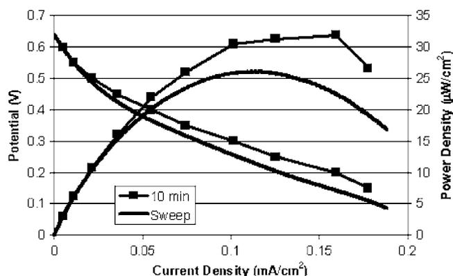
**Figure 11.** Comparison between steady state (at 10 min) and linear voltammetry polarization data for sample D with humidified hydrogen at room temperature.
