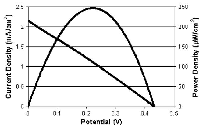
**Figure 12.** Microchannel full cell performance with 1.0 M acidic methanol at 1 mL/h.
