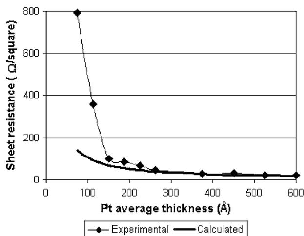
Figure 3. Measured and calculated resistances for sputtered platinum films.
