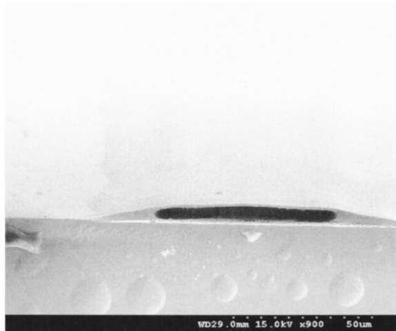
Fig. 8. Example of an air channel fabricated using Unity2203P as a sacrificial polymer and \sim 1 \mu\text{m} thick \text{SiO}_2 as an overcoat layer.
