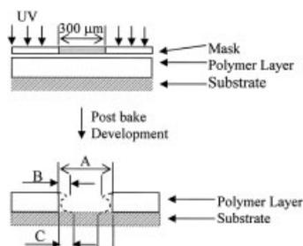
**Figure 3** Illustration of via-hole formed in polymer film.
