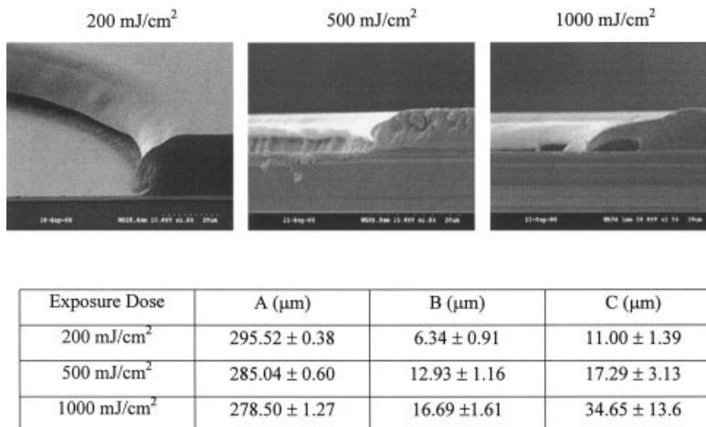
**Figure 6** SEM pictures of the via-holes opened in 40/60 polymer films (formulation II) exposed to 200, 500, and 1000 mJ/cm<sup>2</sup> doses.
