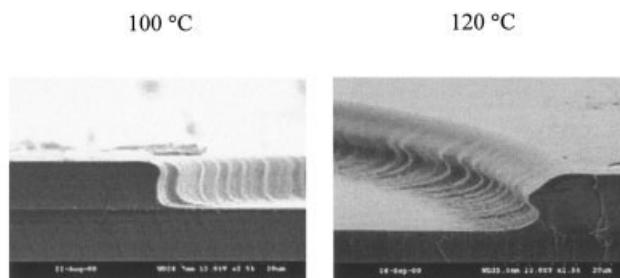
**Figure 7** SEM pictures of the via-holes opened in 40/60 polymer films (formulation II) post-exposure baked at 100°C and 120°C.
