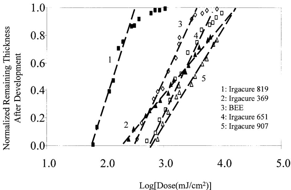
Figure 4 Contrast curves for photosensitive PNB formulations with various PIs at the same loading of 0.32 wt %.
