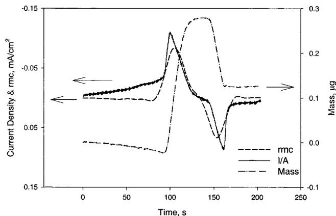
**Figure 5.** CV of aluminum in LiTFSI-EMSF with mass change and *rmc*. Switching potential was 0 V. Area of WE is 0.385 cm<sup>2</sup>.
