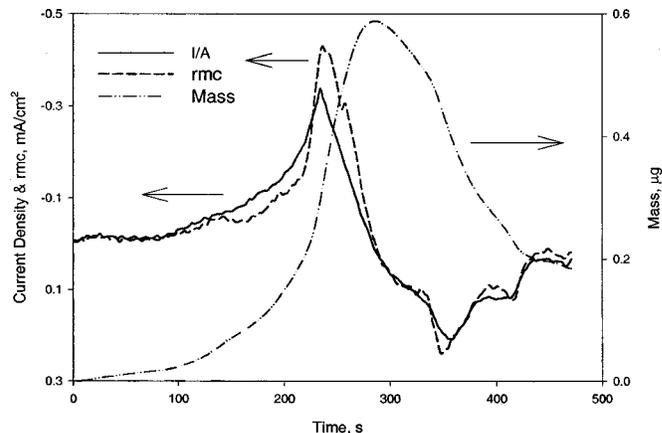
**Figure 2.** CV of platinum in LiTFSI-EMSF with mass change and *rmc*. Area of WE is  $0.252 \text{ cm}^2$ .
