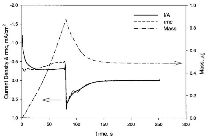
**Figure 4.** CA of platinum in LiTFSI-EMSF with mass change and *rmc*. Reduction potential was  $-0.3$  V. Area of WE is 0.252 cm<sup>2</sup>.
