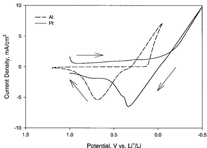
**Figure 1.** CVs of aluminum and platinum in LiTFSI-EMSF. Area of the Al WE is  $0.0785 \text{ cm}^2$ . Area of Pt WE is  $0.158 \text{ cm}^2$ .
