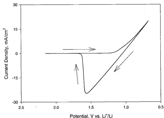
**Figure 8.** CV of Hg electrode in LiTFSI-EMSF. Area of WE is  $0.318 \text{ cm}^2$ .
