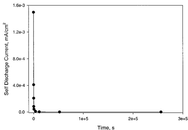
**Figure 7.** Self-discharge rate of lithium on aluminum substrate.
