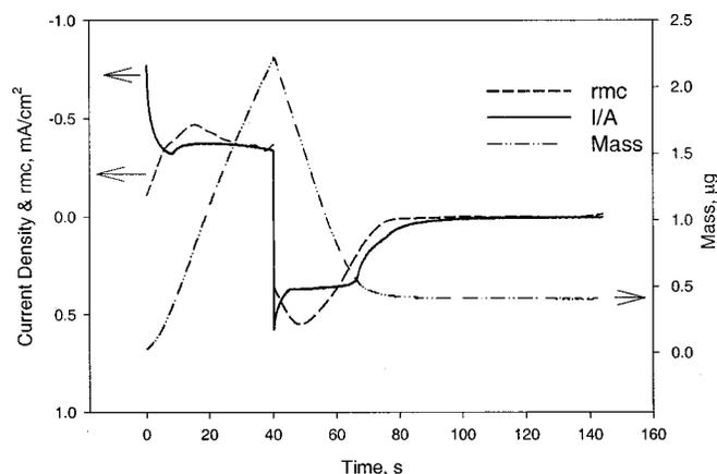
**Figure 6.** CA of aluminum in LiTFSI-EMSF with mass change and  $rmc$ . Area of WE is  $0.385 \text{ cm}^2$ .
