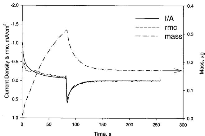
**Figure 3.** CA of platinum in LiTFSI-EMSF with mass change and *rmc*. Reduction potential was 0 V. Area of WE is 0.252 cm<sup>2</sup>.
