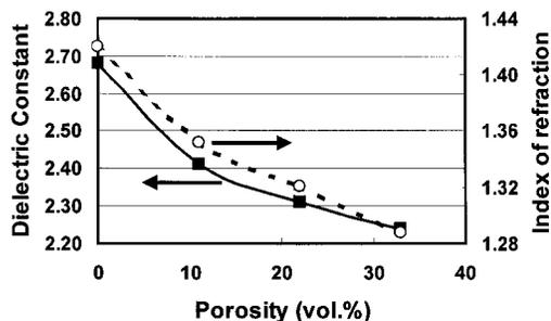
Figure 2. Measured dielectric constant and index of refraction as a function of the estimated porosity in the films.
