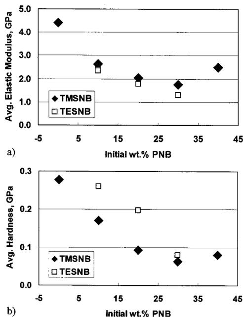
**Figure 5.** Plot of (a) average elastic modulus, and (b) average hardness as a function of the initial weight percent of TMSNB or TESNB in the films.
