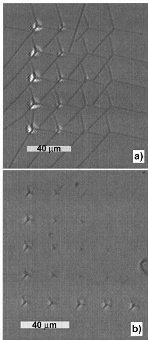
Figure 3. Fracture toughness indents for an (a) MSQ film and (b) 10:90 wt % TESNB:MSQ film.
