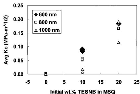
Figure 4. Plot of the average fracture toughness as a function of the initial weight percent of TESNB in the film and the average thickness.
