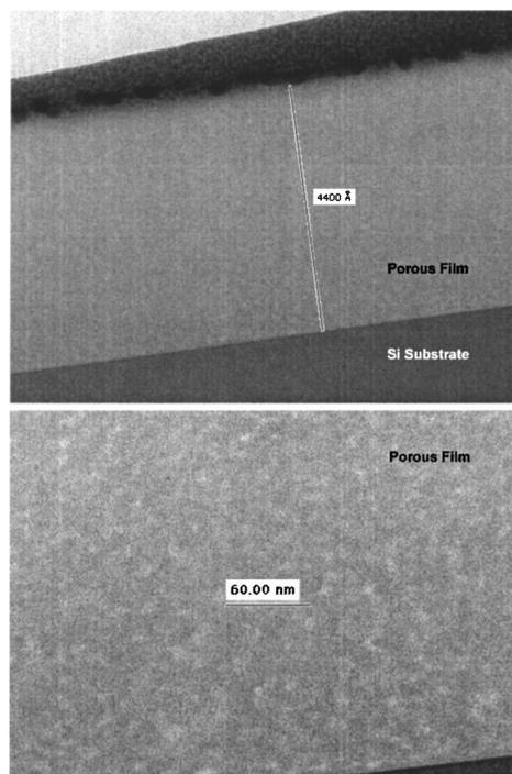
Figure 1. TEM images for a 20:80 wt % TMSNB:MSQ film after decomposition.
