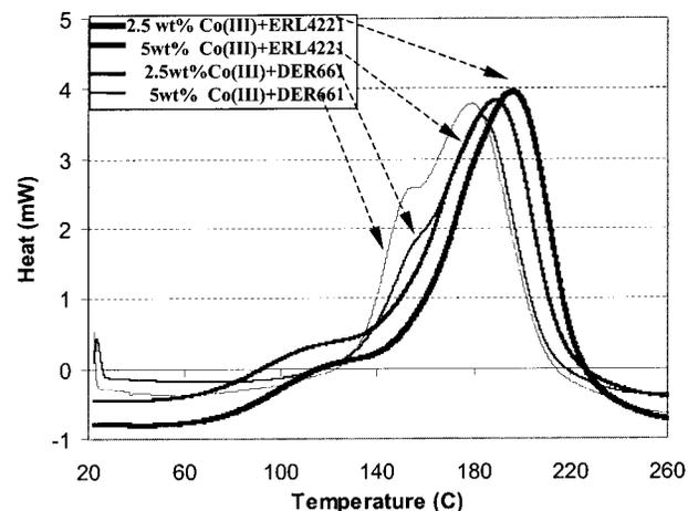
**Figure 7** DSC curves of different epoxy formulations.
