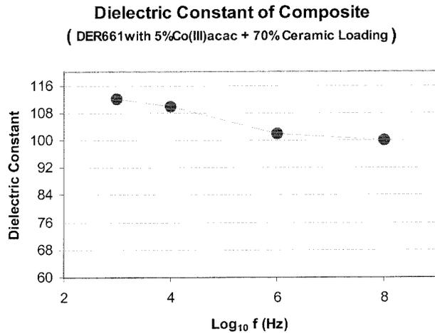
**Figure 10** Dielectric constant of composite at different frequencies.
