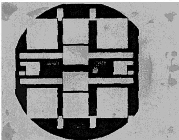
**Figure 4** Prototype of capacitors fabricated by thick-film technology.
