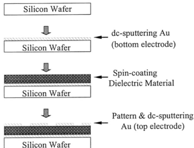
**Figure 5** Fabrication process of prototype of embedded capacitors.
