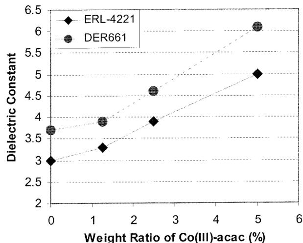
**Figure 8** Dielectric constant of epoxy systems with Co(III)–acac.
