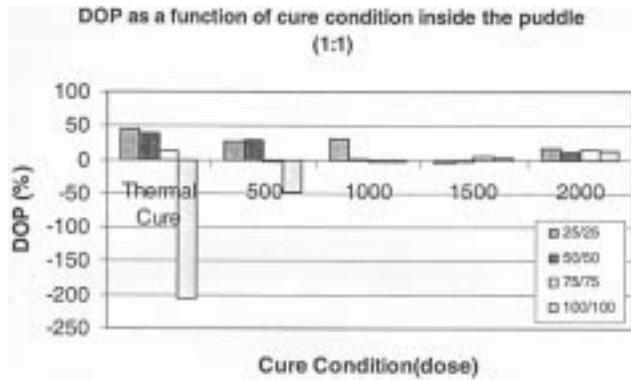
Fig. 8. Degree of planarization as a function of cure condition for features (1 : 1) inside the puddle (average height of metal line  $2.5 \mu\text{m}$ ).
