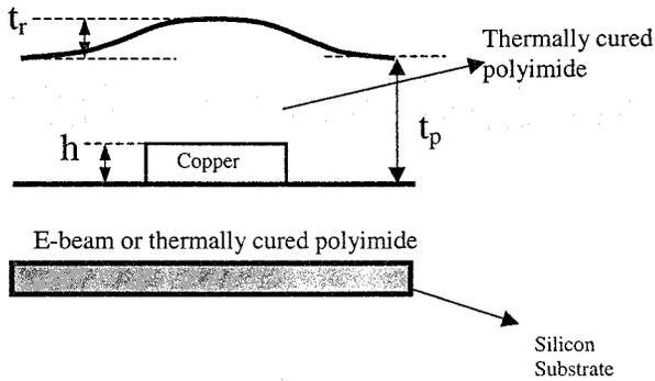
Fig. 1. Definition of degree of planarization (DOP) in a multilayer structure  $h$  = height of copper metal line,  $t_p$  = thickness of polymer,  $t_r$  = relief height of polymer over metal line.
