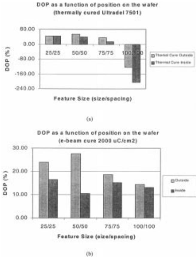
Fig. 12. Degree of planarization as a function of feature location on the wafer (a) thermally cured base (b) e-beam cured base cured with a dose of 2000  $\mu\text{C}/\text{cm}^2$ .
