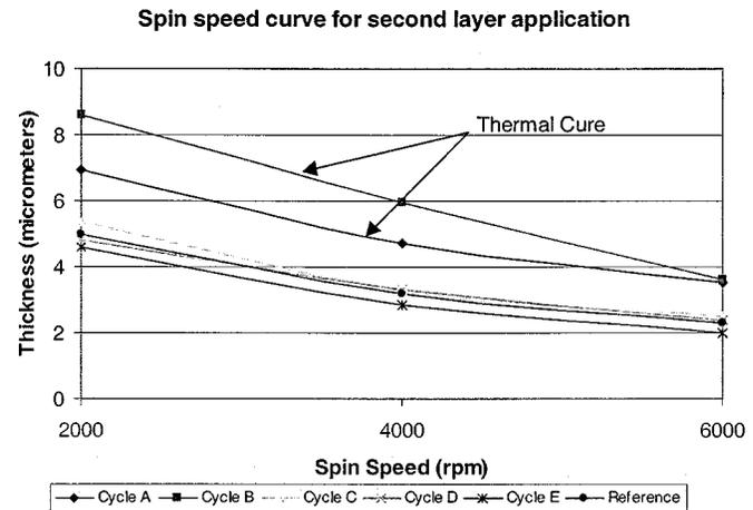
Fig. 3. Spin speed curve for second layer of polyimide spun over polyimide base cured under various conditions.
