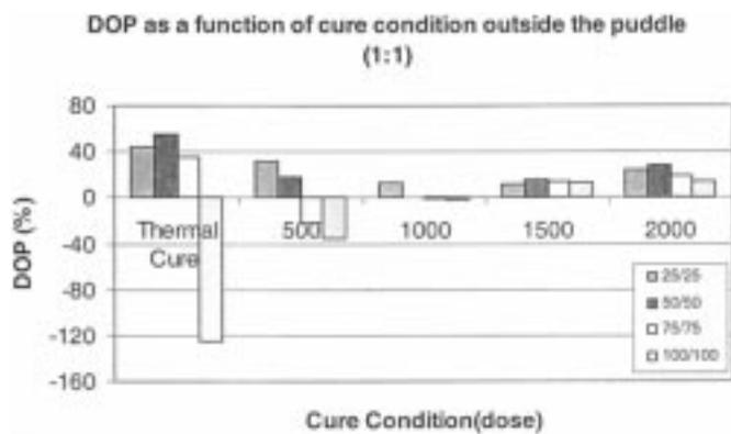
Fig. 6. Degree of planarization as a function of cure condition for features (1 : 1) outside the puddle (average height of metal line 2.5  $\mu\text{m}$ ).
