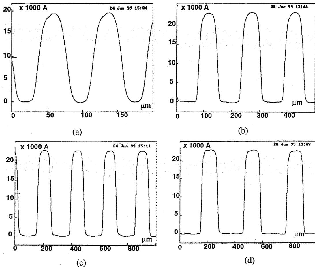
Fig. 5. Surface topography scan of polymer on top a metal line, with an e-beam cured base with a width/spacing ratio of (a) 25  $\mu\text{m}/50 \mu\text{m}$ , (b) 50  $\mu\text{m}/100 \mu\text{m}$ , (c) 75  $\mu\text{m}/150 \mu\text{m}$ , and (d) 100  $\mu\text{m}/200 \mu\text{m}$  feature size (average height of metal line 2.5  $\mu\text{m}$ ).
