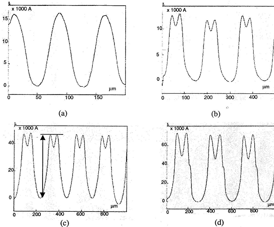
Fig. 4. Surface topography scan of polymer on top a metal line, with a thermally cured base with a width/spacing ratio of (a)  $25\ \mu\text{m}/50\ \mu\text{m}$ , (b)  $50\ \mu\text{m}/100\ \mu\text{m}$  (c)  $75\ \mu\text{m}/150\ \mu\text{m}$  and (d)  $100\ \mu\text{m}/200\ \mu\text{m}$  feature size (average height of metal line  $2.5\ \mu\text{m}$ ).
