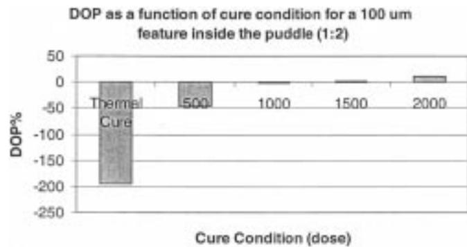
Fig. 11. DOP as a function of cure condition for a 100  $\mu\text{m}$  feature inside the puddle with 200  $\mu\text{m}$  spacing between lines.
