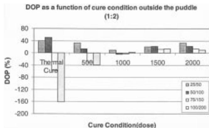
Fig. 7. Degree of planarization as a function of cure condition for features (1 : 2) outside the puddle (average height of metal line 2.5  $\mu\text{m}$ ).
