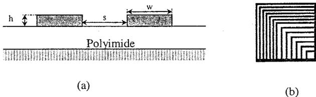
Fig. 2. Test structure for characterization of degree of planarization: (a) schematic side view, (b) top view of a single structure, and (c) schematic view of the wafer.
