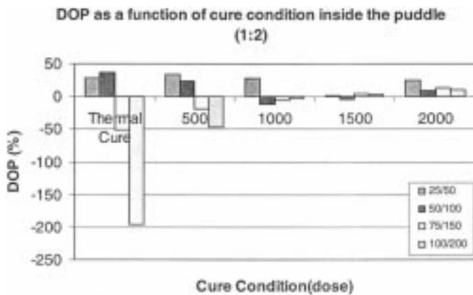
Fig. 9. Degree of planarization as a function of cure condition for features (1 : 2) inside the puddle (average height of metal line  $2.5 \mu\text{m}$ ).
