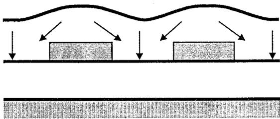
Fig. 10. Solvent redistribution from second layer of polymer leading to solvent swelling effects.
