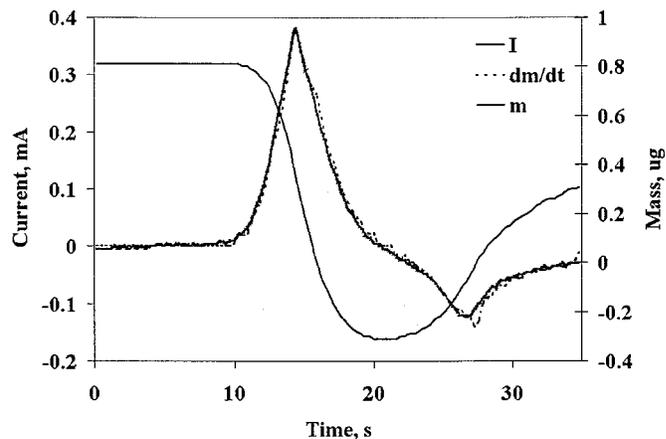
**Figure 9.** CV of copper-plated Pt quartz crystal using the EQCN. Electrode area is  $0.196 \text{ cm}^2$ .
