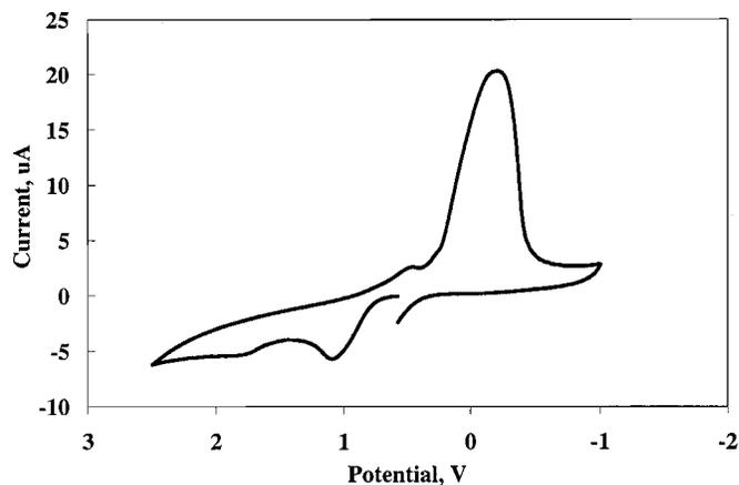
Figure 2. CV of Cu in 35/65 MSC melt. Scan started in the positive direction showing oxidation then reduction. Electrode area is  $0.0079 \text{ cm}^2$ .
