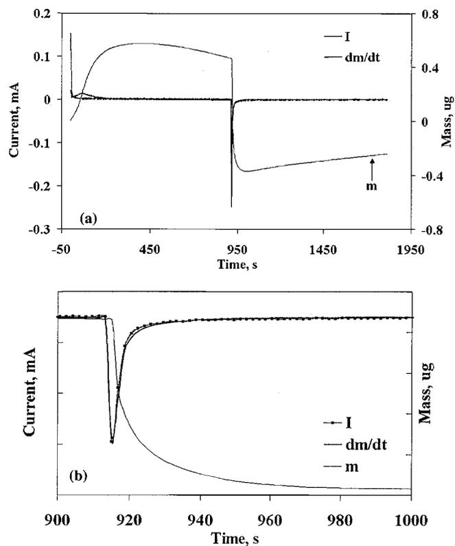
**Figure 10.** (a, top) CA of copper-plated Pt quartz crystal using the EQCN. (b, bottom) Shows the first 100 s of reduction step. Electrode area is  $0.196 \text{ cm}^2$ .
