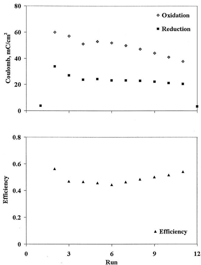
**Figure 7.** Plot of CA results of copper-plated electrode in supernatant above NaCl slurry showing more reduction than oxidation.
