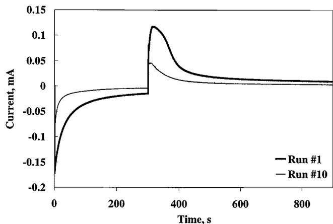
Figure 4. CA of a copper-plated electrode submerged in supernatant above NaCl slurry. Electrode area is 0.158 cm<sup>2</sup>.
