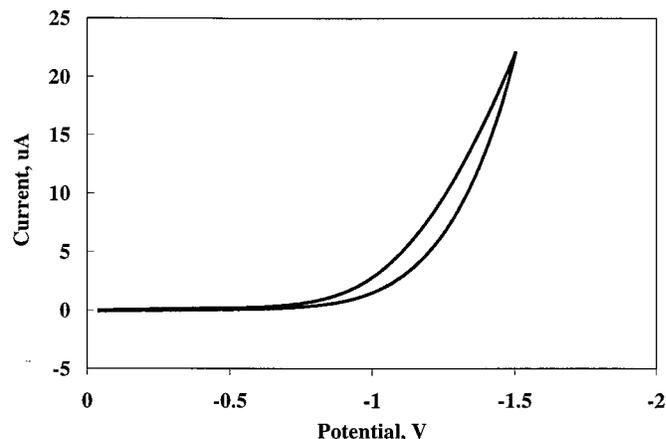
Figure 3. CV of Cu in 35/65 MSC melt. The scan started in the negative direction showing no reduction. Electrode area is  $0.0079 \text{ cm}^2$ .
