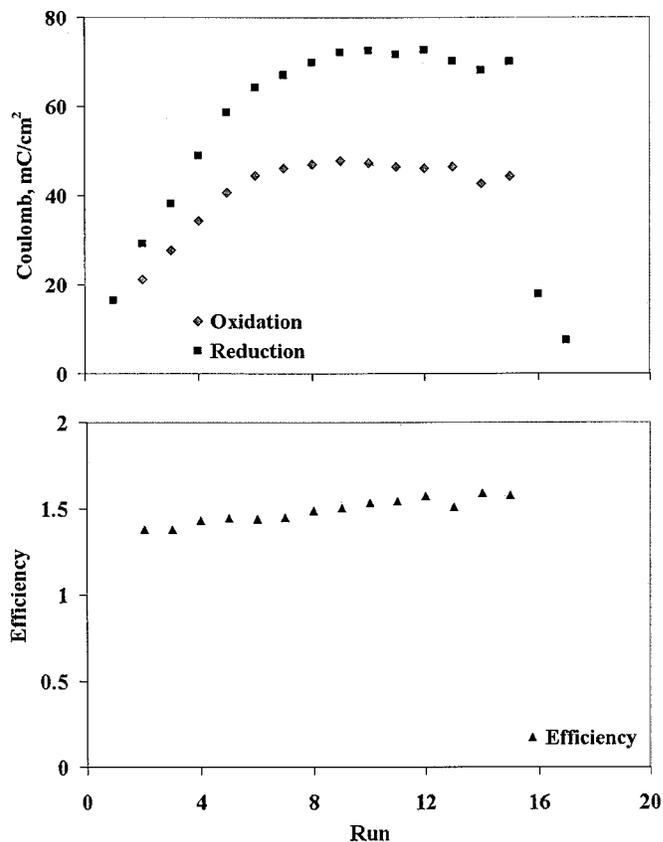
**Figure 8.** Plot of CA results of solid copper electrode with steady oxidation and reduction.
