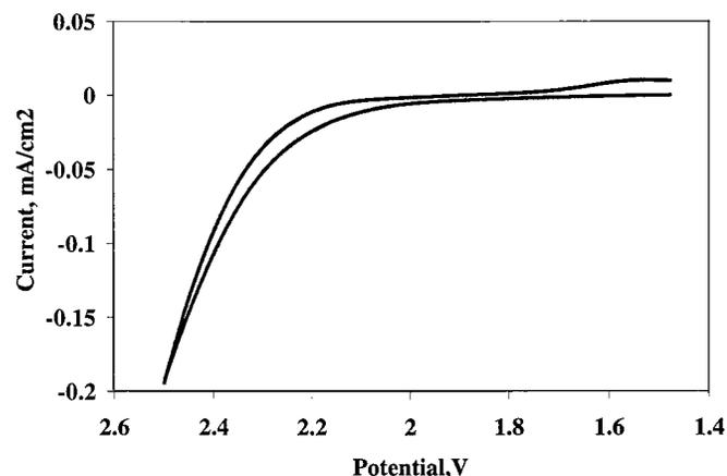
Figure 1. CV of platinum in 35/65 MSC melt showing the positive end of electrochemical window of melt.
