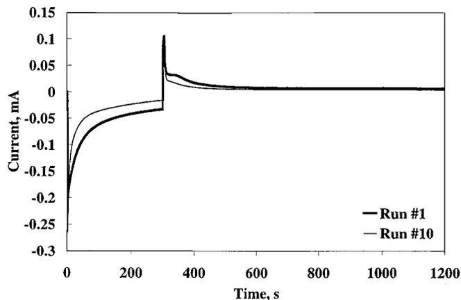
Figure 5. CA of a copper-plated electrode submerged in NaCl slurry. Electrode area is 0.158 cm<sup>2</sup>.
