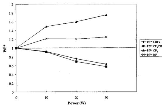
Fig. 6. Plot of  $P/P^*$  vs applied power (W).  $P^*$  and  $P$  refer to the partial pressure of a particular mass spectrometer fragment before and 5 min after plasma ignition, respectively. Substrate temperature: 120 °C, operating pressure: 1 Torr.
