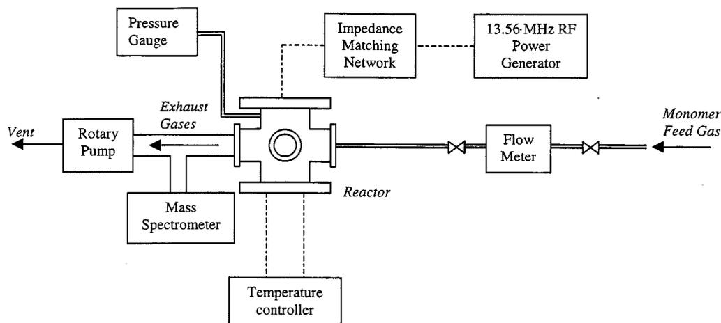
FIG. 1. Schematic of the parallel plate plasma reactor system used for fluoropolymer film deposition.
