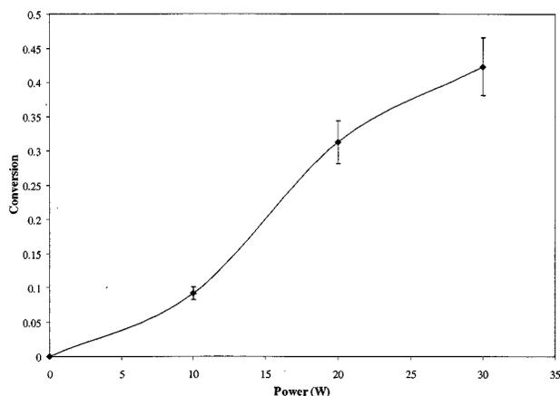
FIG. 7. Monomer conversion as a function of applied power (W). Note that, conversion refers to the fraction of the monomer fragmented in the plasma. Substrate temperature: 120 °C, operating pressure: 1 Torr.
