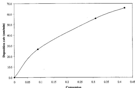
FIG. 8. Polymer deposition rate (nm/min) as a function of monomer conversion. Substrate temperature: 120 °C, operating pressure: 1 Torr.
