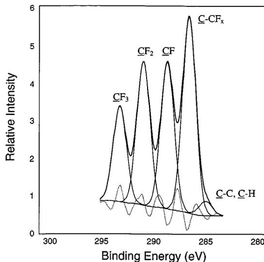
FIG. 3. High-resolution C 1s spectrum of a polymer film obtained by XPS analysis at a pass energy of 11.75 eV. Deposition conditions: 30 W, 120 °C, 1 Torr.
