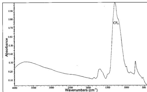
Fig. 5. Infrared spectrum of a deposited polymer film. Deposition conditions: 20 W, 120 °C, 1 Torr, 1 h.
