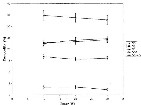
FIG. 4. XPS composition (%) of  $\text{CF}_3$ ,  $\text{CF}_2$ ,  $\text{CF}$ ,  $\text{C-CF}_x$ , and  $\text{C-C}$  or  $\text{C-H}$  in a deposited polymer film as a function of applied power (W). Substrate temperature: 120 °C, total pressure: 1 Torr.
