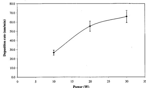
FIG. 2. Deposition rate (nm/min) as a function of applied power (W) at a total pressure of 1 Torr and 120 °C substrate temperature.
