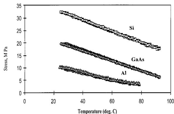
**Figure 1.** Stress as a function of temperature for approximately 14.6  $\mu\text{m}$  thick Cyclotene.
