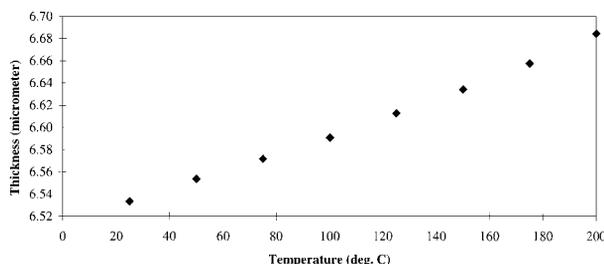
**Figure 4.** Film thickness as a function of temperature calculated from comb electrode in Figure 3.
