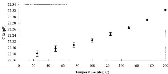
**Figure 9.** Interelectrode capacitance as a function of temperature for bare chrome-on-glass comb electrode.
