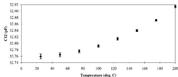
**Figure 6.** Interelectrode capacitance for chrome-on-glass comb electrode coated with  $6.5 \mu\text{m}$  Cyclotene film. Same electrode as in Figure 5.
