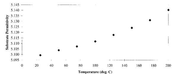
**Figure 11.** Permittivity of the glass substrate calculated from data in Figure 9.
