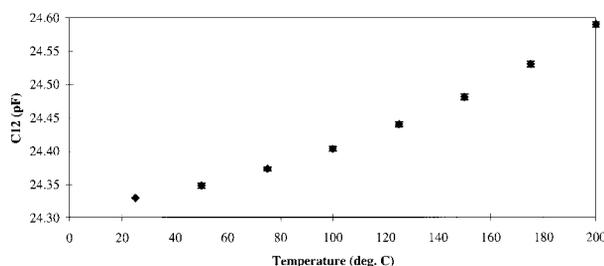
**Figure 5.** Interelectrode capacitance of a bare chrome-on-glass comb electrode as a function of temperature.
