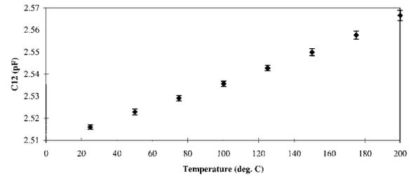
**Figure 3.** Interelectrode capacitance for 10  $\mu\text{m}$  line/space comb electrode fabricated on 6.5  $\mu\text{m}$  thick Cyclotene.
