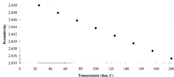
**Figure 12.** Permittivity as a function of temperature of 1.2  $\mu\text{m}$  thick Cyclotene film calculated using data in Figure 10.
