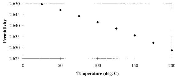
**Figure 8.** Permittivity as a function of temperature for 6.5  $\mu\text{m}$  thick Cyclotene, determined using chrome-on-glass comb electrode.
