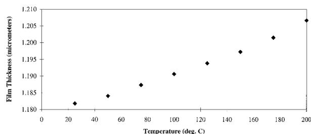
**Figure 13.** Cyclotene film thickness as a function of temperature determined using chrome-on-glass comb electrode and parallel-plate capacitor data.
