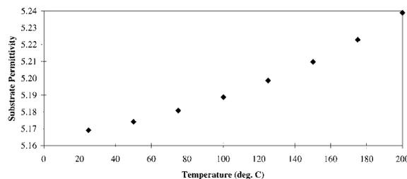
**Figure 7.** Permittivity of glass substrate determined from data of bare chrome-on-glass sensor in Figure 5.
