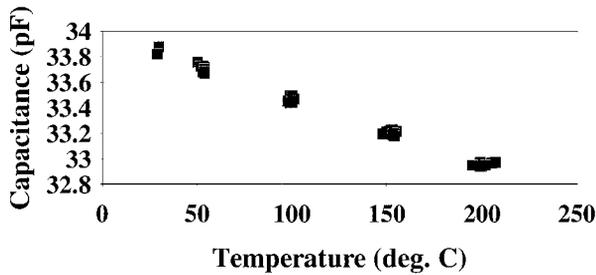
**Figure 2.** Capacitance as a function of temperature as determined from parallel plate capacitor measurements for a 30  $\mu\text{m}$  Cyclotene film.
