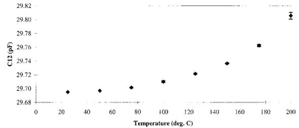
**Figure 10.** Interelectrode capacitance as a function of temperature for chrome-on-glass comb electrode coated with 1.2  $\mu\text{m}$  thick Cyclotene. Same electrode as Figure 9.
