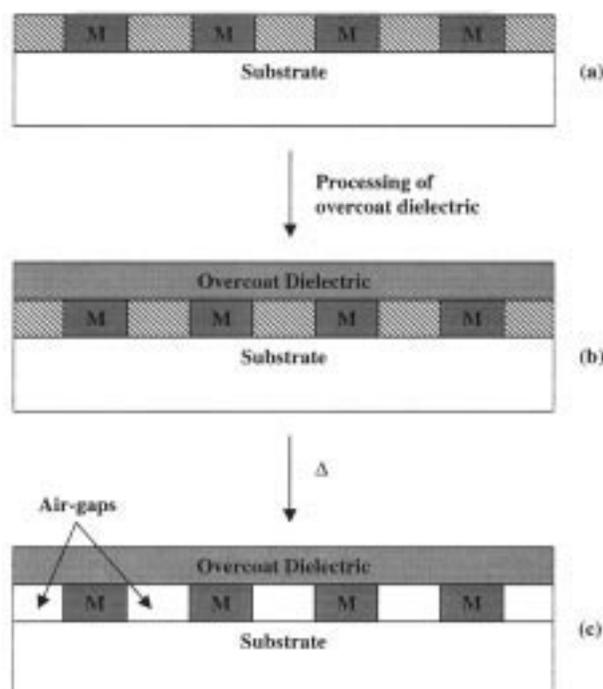
**Figure 1.** Diagram of air-gap structure. (a) The sacrificial layer is formed between metal lines (M). (b) An overcoat dielectric layer is deposited over the metal/sacrificial polymer layer. (c) The air-gap is formed by decomposing the sacrificial polymer.
