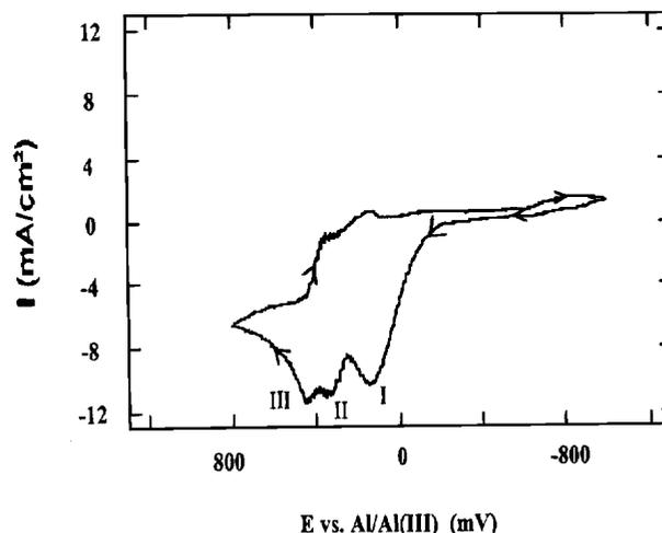
Fig. 2. Cyclic voltammogram of iron disk electrode in basic (*N* = 0.45) MEIC:AlCl<sub>3</sub> at room temperature. Scan rate 100 mV/s and electrode area 7.85 × 10<sup>-3</sup> cm<sup>2</sup>.
