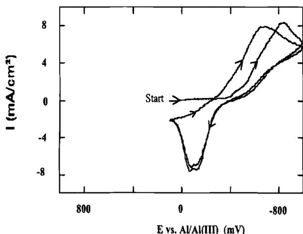
Fig. 3. Cyclic voltammogram at platinum coil electrode in a neutral-like MEIC: $\text{AlCl}_3$  melt at  $70^\circ\text{C}$ . Scan rate 50 mV/s and electrode area  $0.4$  cm<sup>2</sup>.
