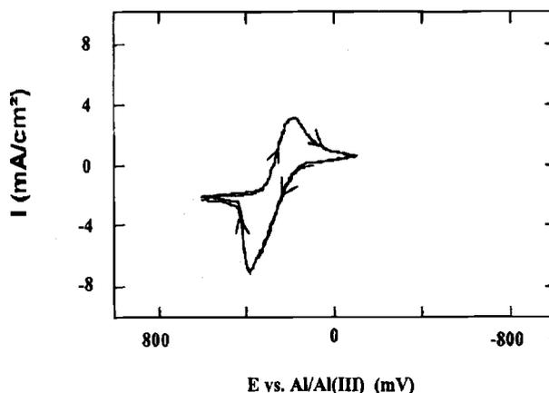
Fig. 4. Cyclic voltammogram at platinum coil electrode in a neutral-like MEIC: $\text{AlCl}_3$  melt at  $70^\circ\text{C}$ . Scan rate 50 mV/s and electrode area  $0.4$  cm<sup>2</sup>.
