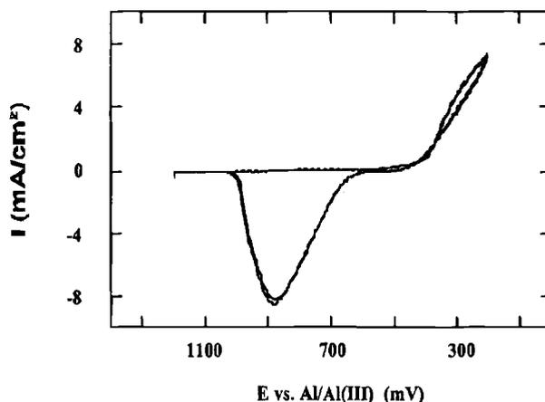
Fig. 5. Cyclic voltammogram at platinum coil electrode in acidic ( $N = 0.55$ ) MEIC: $\text{AlCl}_3$  melt with 26 mM  $\text{FeCl}_2$  at room temperature. Scan rate 50 mV/s and electrode area  $0.4$  cm<sup>2</sup>.
