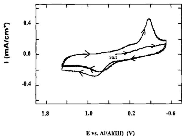
Fig. 8. Cyclic voltammogram consisting of three cycles of a nickel wire electrode in NaCl-buffered, neutral MEIC:AlCl<sub>3</sub> at 20°C. Scan rate 100 mV/s and electrode area 0.32 cm<sup>2</sup>.
