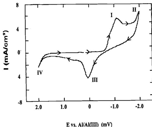
Fig. 6. Cyclic voltammogram at iron/iron(III) chloride wire electrode in NaCl-buffered, neutral MEIC:AlCl<sub>3</sub> melt at room temperature. Scan rate 100 mV/s and electrode area 0.071 cm<sup>2</sup>.
