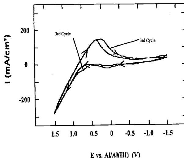
Fig. 7. Cyclic voltammogram consisting of three cycles of a copper disk electrode in NaCl-buffered, neutral MEIC:AlCl<sub>3</sub> at room temperature. Scan rate 1 V/s and electrode area 7.85 × 10<sup>-3</sup> cm<sup>2</sup>.
