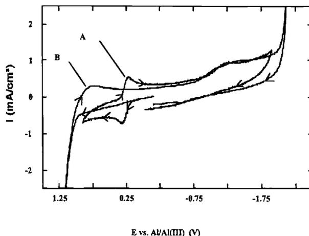
Fig. 1. Cyclic voltammogram at tungsten disk electrode in basic MEIC:AlCl<sub>3</sub> (*N* = 0.48) melt at room temperature with (A) 10 mM FeCl<sub>2</sub> and (B) no FeCl<sub>2</sub>. Scan rate 100 mV/s and electrode area 7.85 × 10<sup>-3</sup> cm<sup>2</sup>.
