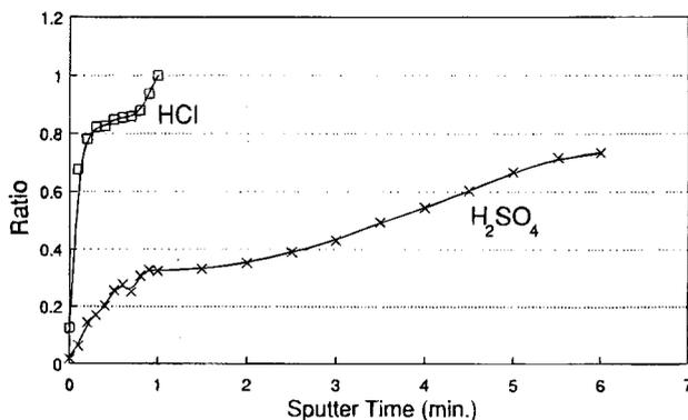
Fig. 4. Ratio of In to As by AES vs. sputter time for n-InAs oxidized in  $0.2\text{M}$  HCl and  $0.2\text{M}$   $\text{H}_2\text{SO}_4$ .
