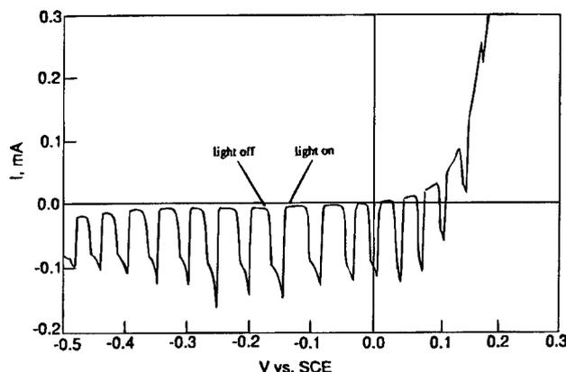
Fig. 3. Photoreduction of p-InAs in 0.2M H<sub>2</sub>SO<sub>4</sub>.
