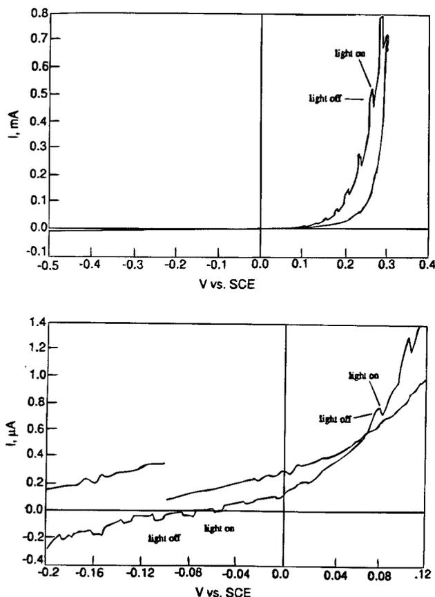
Fig. 2. (a, top) Photo-oxidation of n-InAs in 0.2M H<sub>2</sub>SO<sub>4</sub>; (b, bottom) detail of photoreduction and oxidation.
