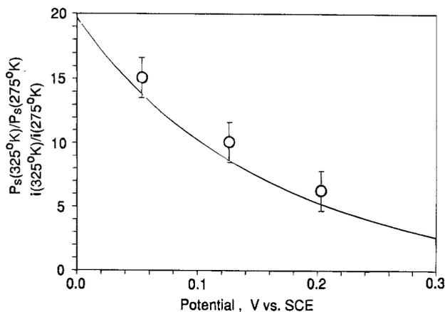
Fig. 5. Ratio of calculated surface hole concentrations 325/275 K (—), ratio of steady-state etch currents 325/275 K (○).
