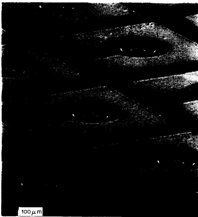
FIG. 2. Scanning electron photomicrograph of a section of an LED wafer with photoelectrochemically etched lenses.
