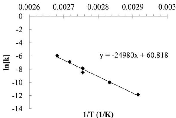
**FIGURE 6** Arrhenius plot for the degradation rate at various isothermals for PPHA.
